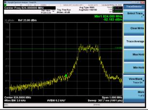
NB-IOT Band 5 QPSK 15kHz 12@0 CH-High
