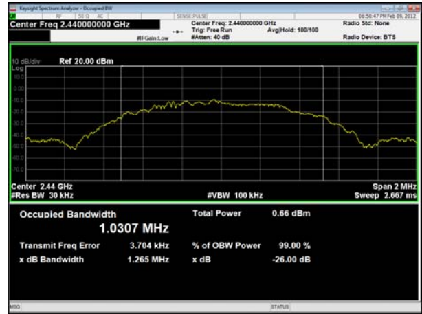
Bluetooth LE Carrier frequency (MHz): 2440
