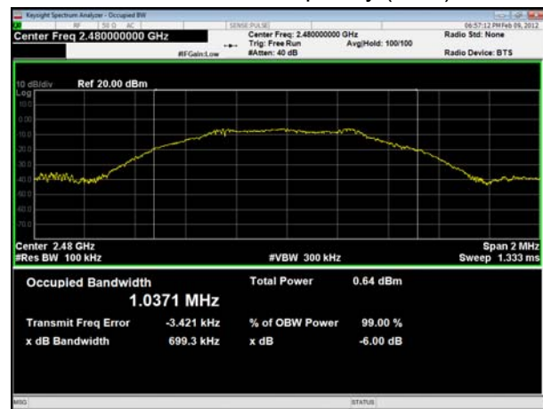
Bluetooth LE Carrier frequency (MHz): 2480
