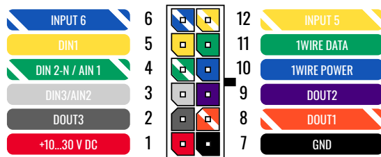
FMM13A 2x6 socket pinout
