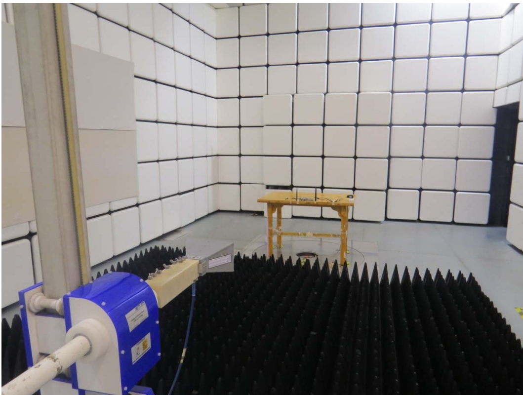
Picture 2: Radiated Spurious Emissions Test setup
