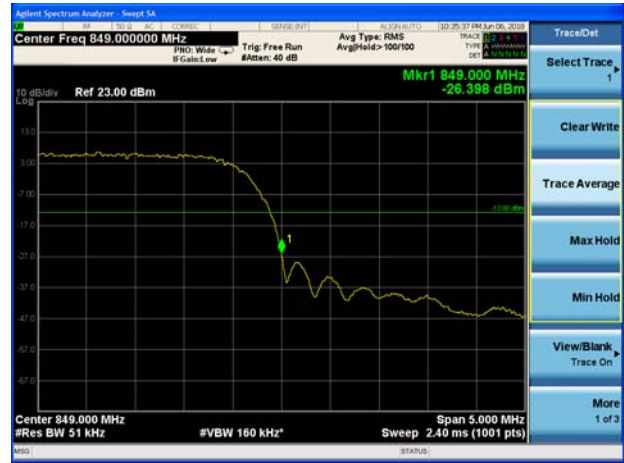
LTE Band 5 QPSK 1.4MHz CH-High 1RB
