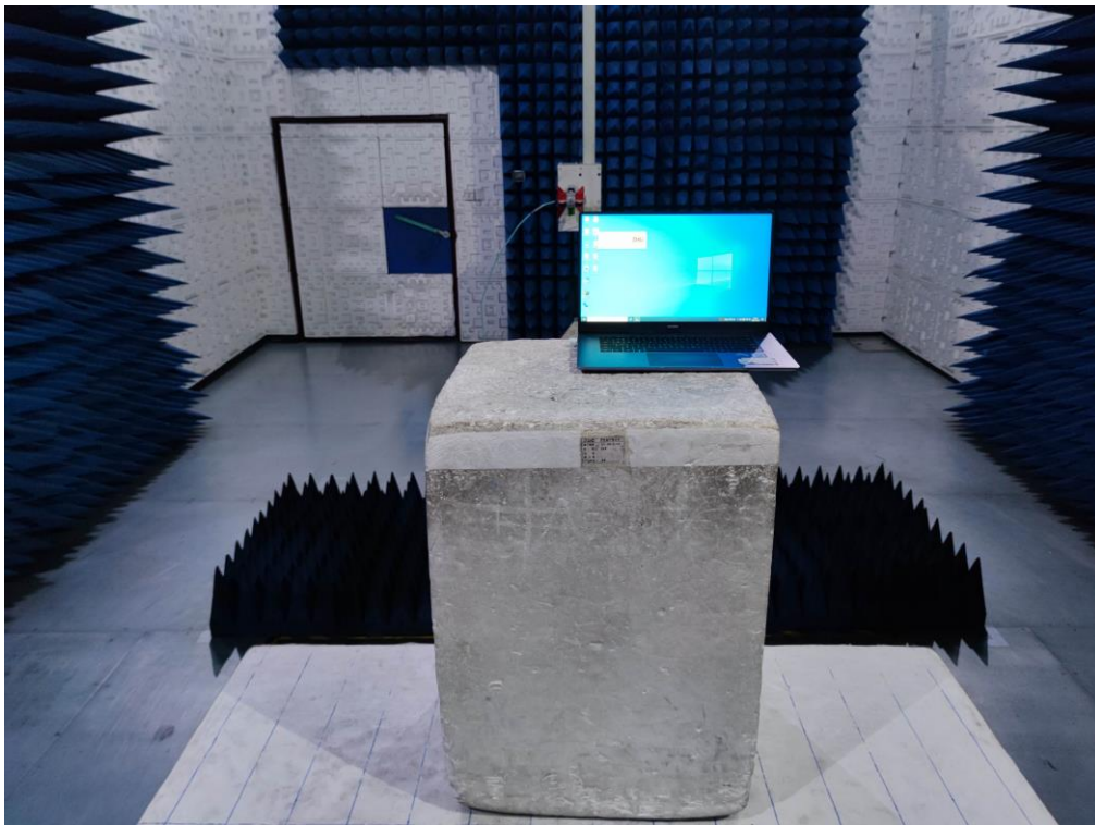
RADIATED EMISSION TEST SETUP ABOVE 1GHz
