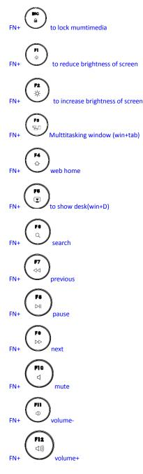
Press F key alone for the corresponding multimedia function, FN + F key to display the function of F key
