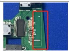
The antenna is PCB antenna. The best case gain of the antenna is 0.11dBi.
