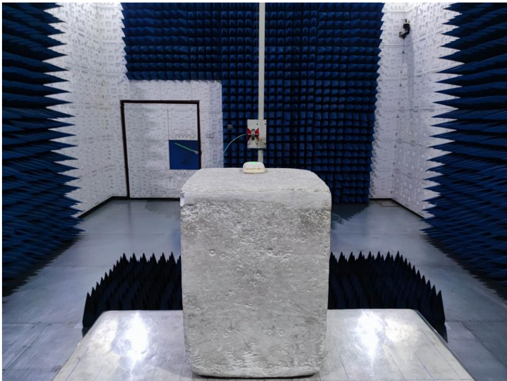
RADIATED EMISSION TEST SETUP ABOVE 1GHz
