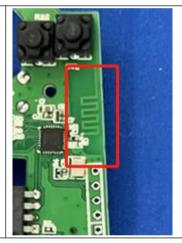
The antenna is PCB antenna. The best case gain of the antenna is -1.52 dBi.
