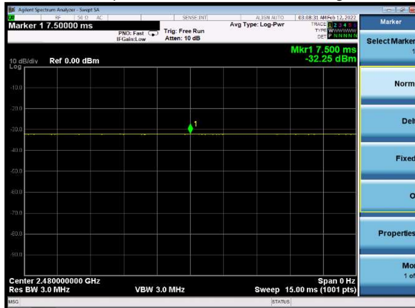
Time-domain plot for Bluetooth transmission signal
