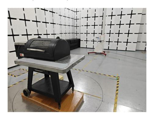
Set-up for Radiated Spurious Emission, Above 1GHz
