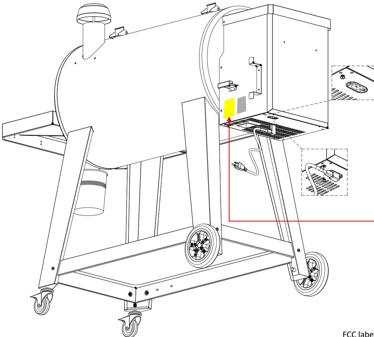
FCC label to be placed on back of the hopper, near the bottom on the left side.
