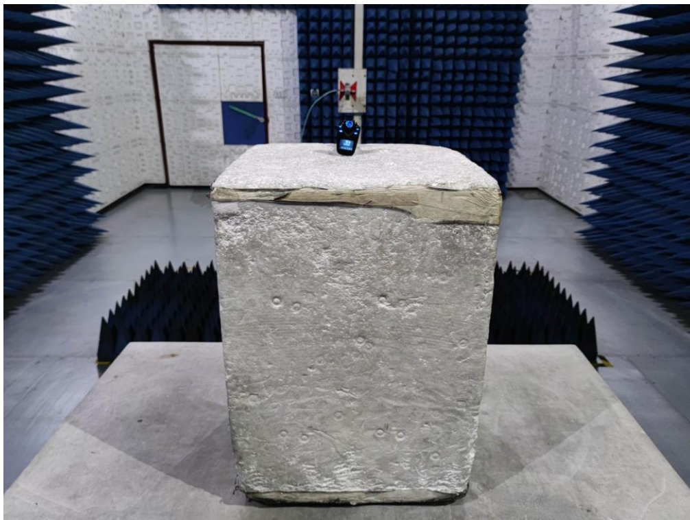
RADIATED EMISSION TEST SETUP ABOVE 1GHz
