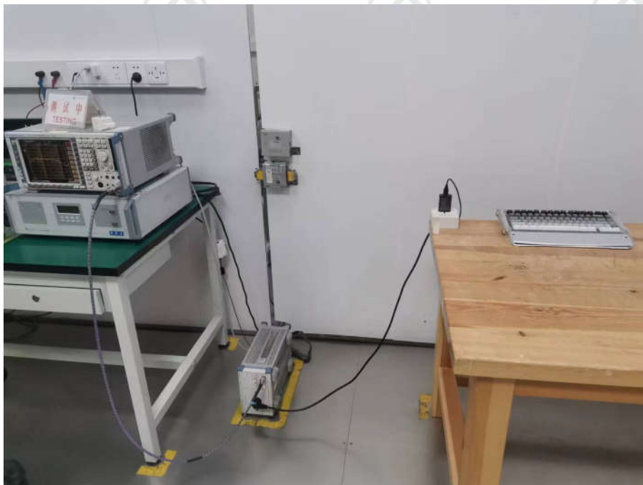
AC Power Line Conducted Emission
