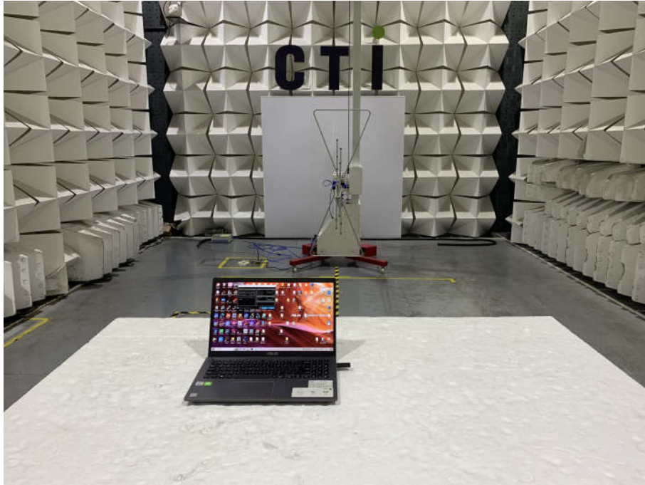
Radiated spurious emission Test Setup-1 (Below 1GHz)
