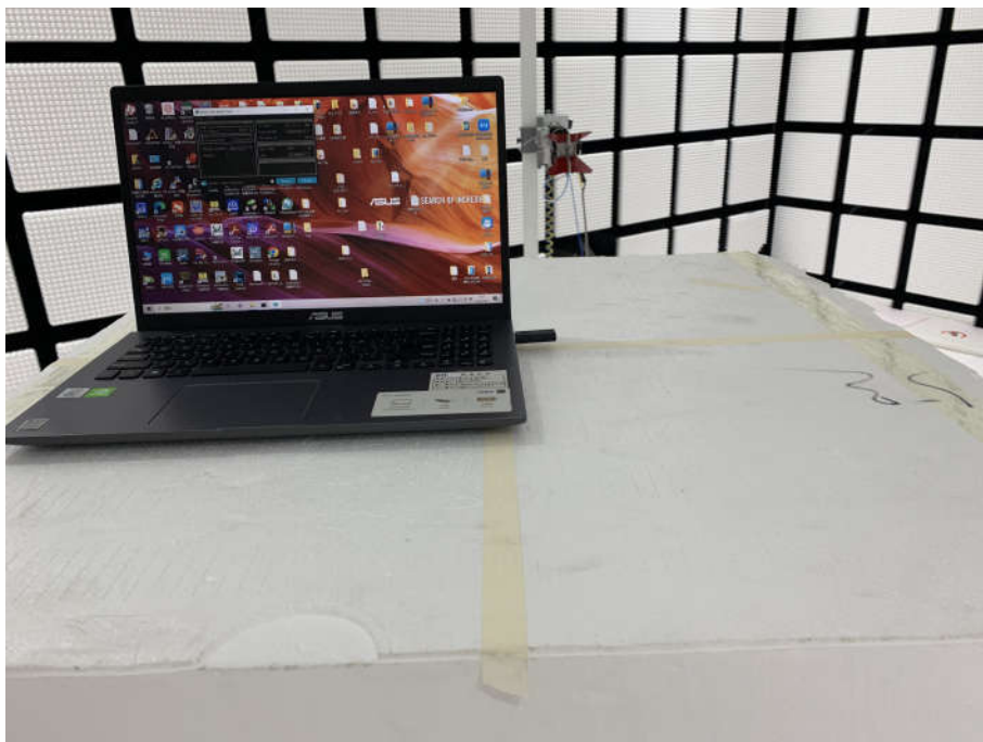
Radiated spurious emission Test Setup-2 (Above 1GHz)
