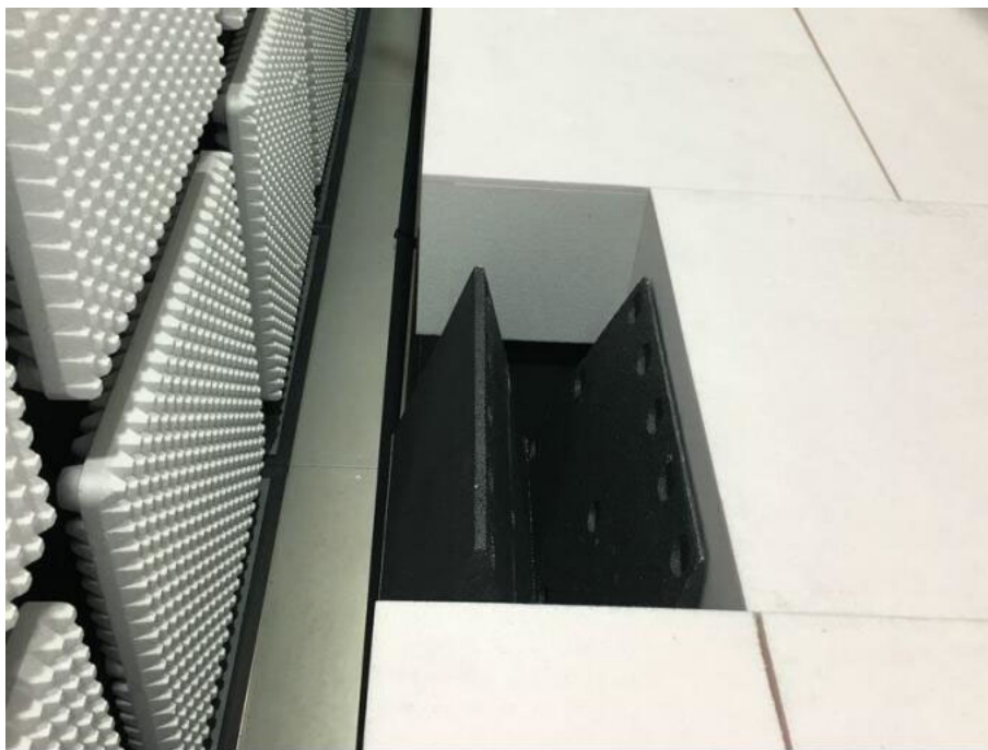
Radiated spurious emission Test Setup-3(Above 1GHz) There are absorbing materials under the ground.
