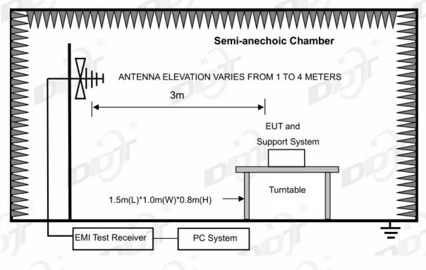
In <u>3 m Anechoic Chamber, test setup diagram for frequency above 1 GHz:</u>
