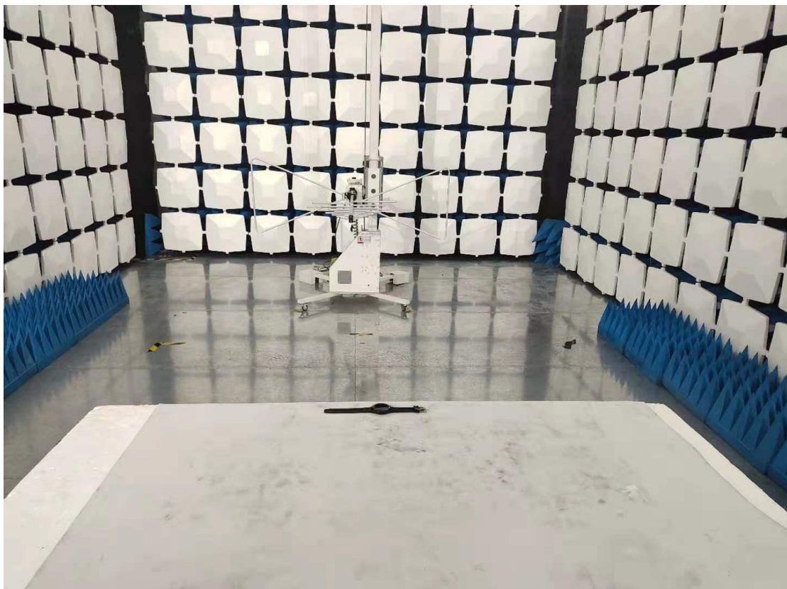
Above 1GHz for radiated emission test setup
