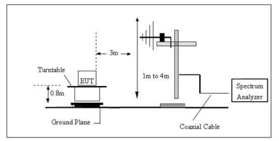
(C) Radiated Emission Test-Up Frequency Above 1GHz
