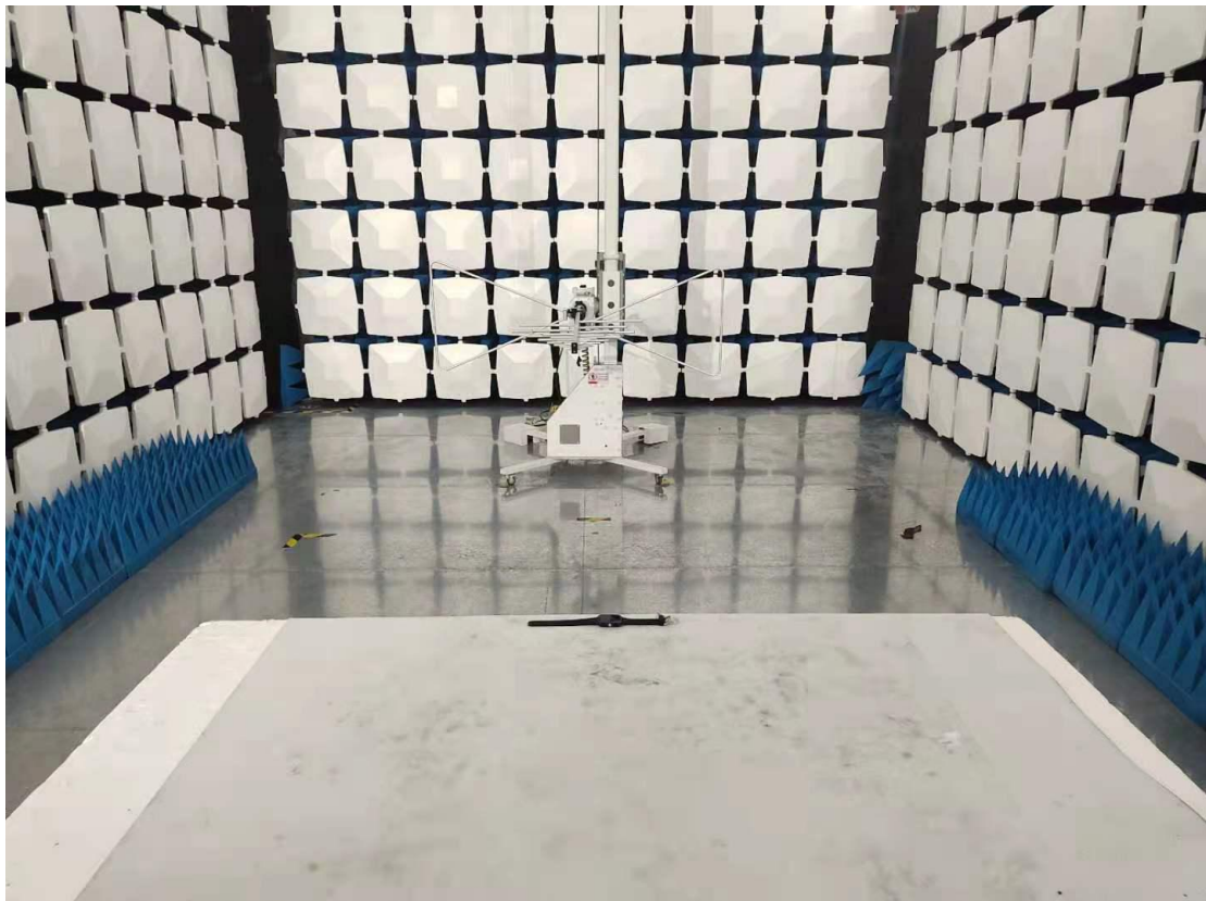
Above 1GHz for radiated emission test setup
