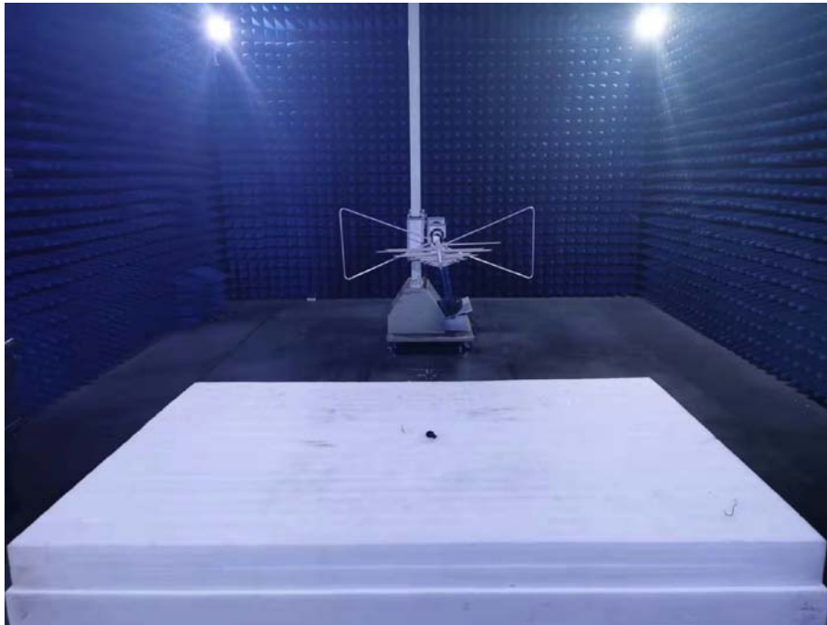
Photo of Radiated Emission Measurement Below 1GHz
