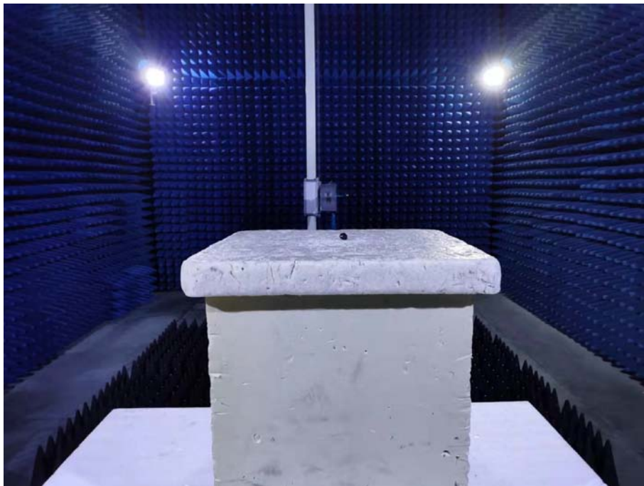
Photo of Radiated Emission Measurement Above 1GHz
