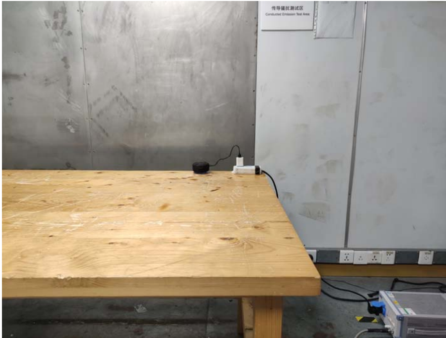
Photo of Power Line Conducted Emission Measurement
