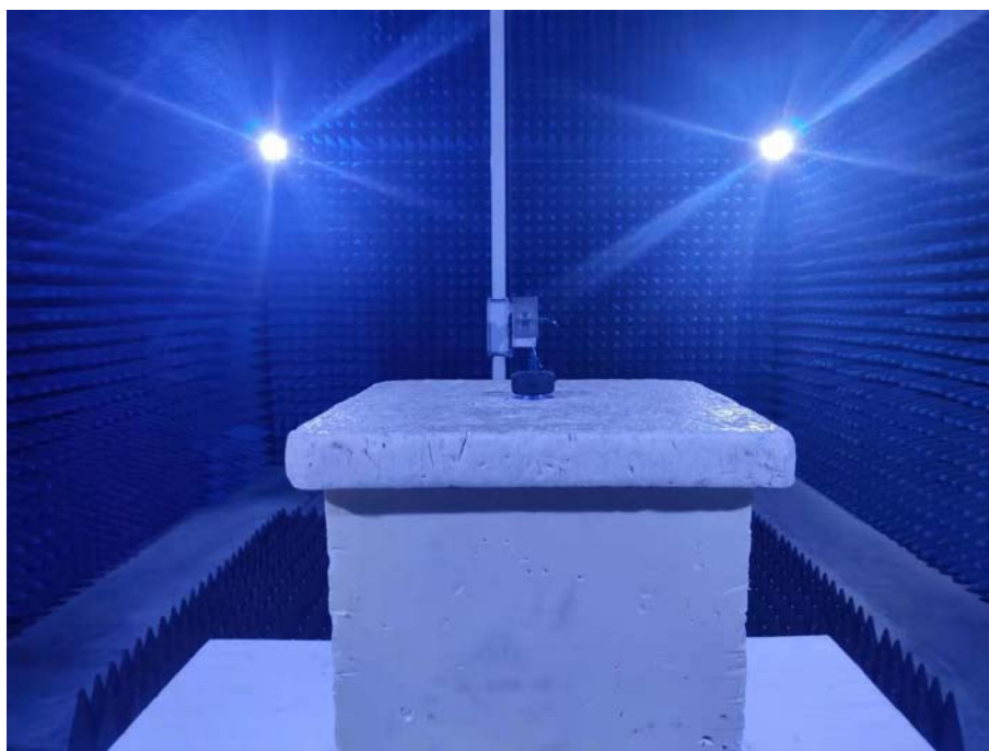
Photo of Radiated Emission Measurement Above 1GHz
