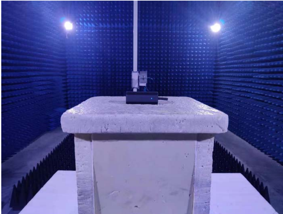
Photo of Radiated Emission Measurement Above 1GHz
