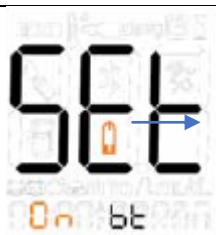
Note: This Bluetooth setting is to set whether to automatically turn on the Bluetooth function after the strip measurement is completed. This can help you to automatically capture your pet's Glucose readings in your AlphaTrak 3 mobile Application. The Bluetooth mode is preset to "OFF".
