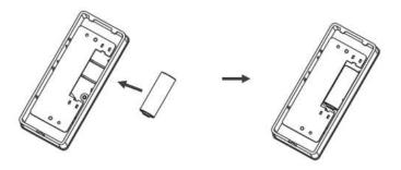
5. Hook the Button with battery onto the wall mounted bottom cover.
