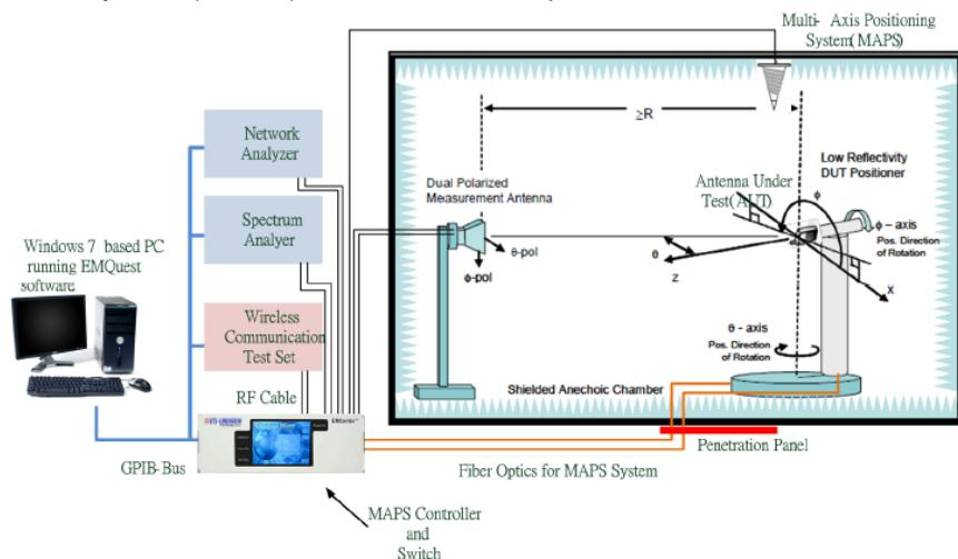
Theta is the spherical axis that rotates along the Cartesian Y axis while Phi is the spherical axis that rotates along the Cartesian Z axis. The initial measurement position (Theta = 0° and Phi = 0°) is illustrated in each of the test setup photographs. The EUT has only one mechanical configuration each and it was tested in the Free-space configuration, whereby the EUT has been placed directly on a support.
