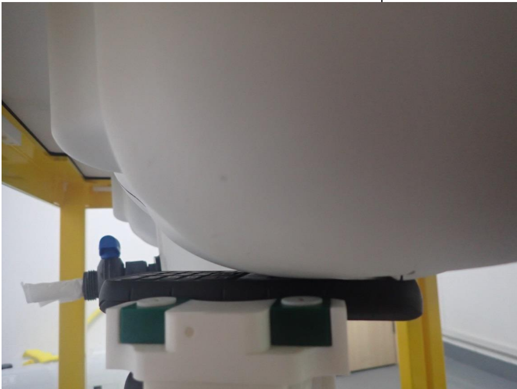
Position of the device under test in relation to the phantom
