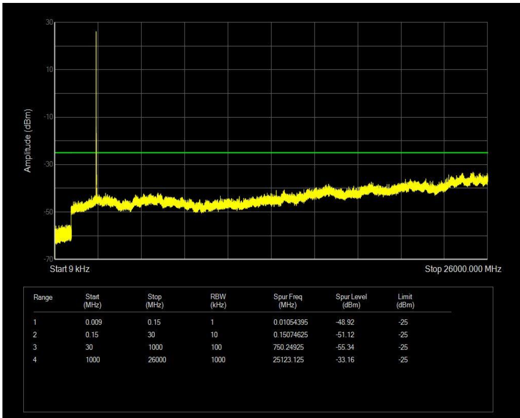
n7 SCS=15kHz CP_QPSK BW=15MHz Channel=501500 RB=1@78
