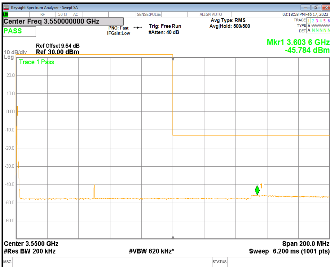
n78(3450-3550) SCS=30kHz CP QPSK BW=100MHz Channel=633332 RB=1@272
