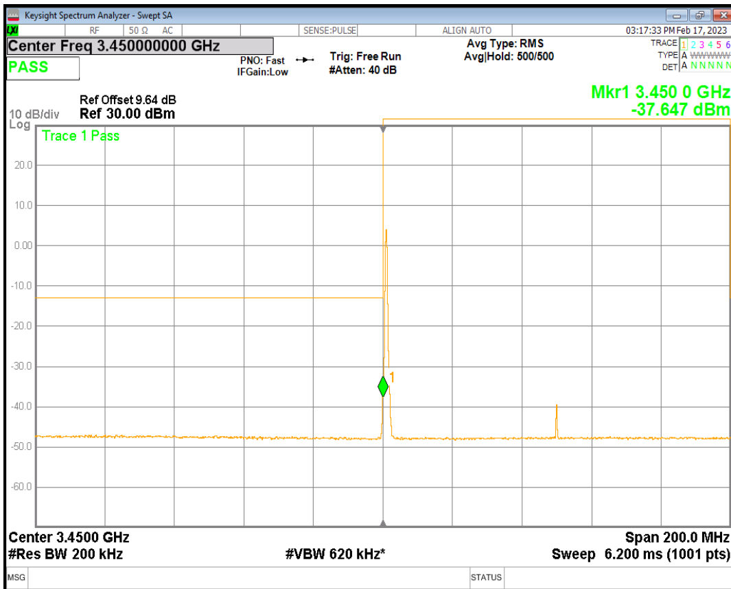
n78(3450-3550) SCS=30kHz CP QPSK BW=100MHz Channel=633334 RB=1@272
