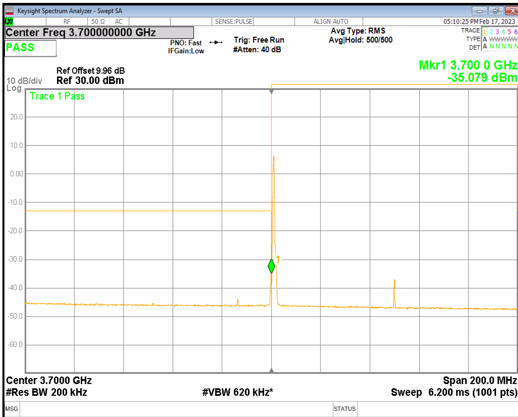
n78(3700-3800) SCS=30kHz CP QPSK BW=100MHz Channel=650000 RB=1@272
