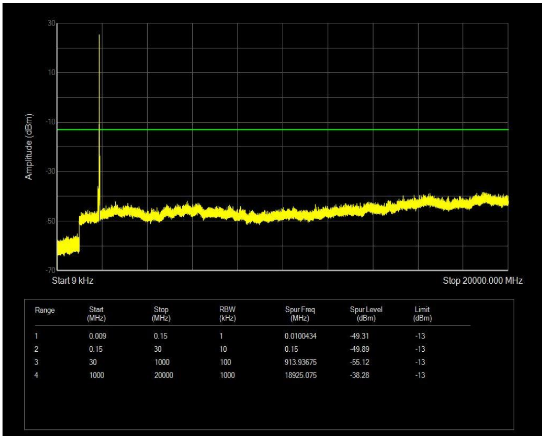
n2 SCS=15kHz CP_QPSK BW=20MHz Channel=380000 RB=1@105
