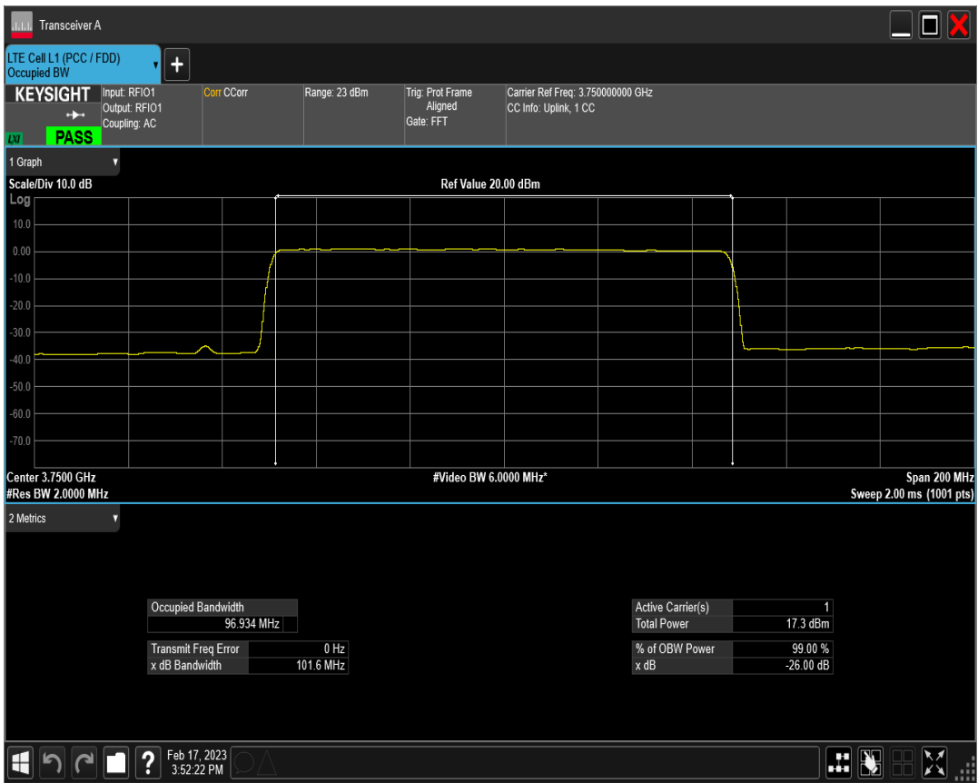
n78(3700-3800) SCS=30kHz DFT 256QAM BW=100MHz Channel=650000 RB=270@0
