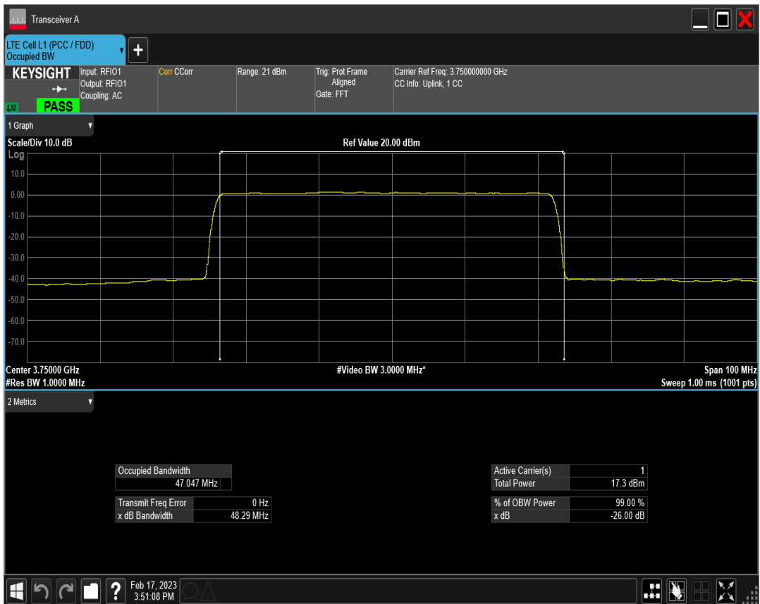
n78(3700-3800) SCS=30kHz DFT 256QAM BW=50MHz Channel=650000 RB=128@0
