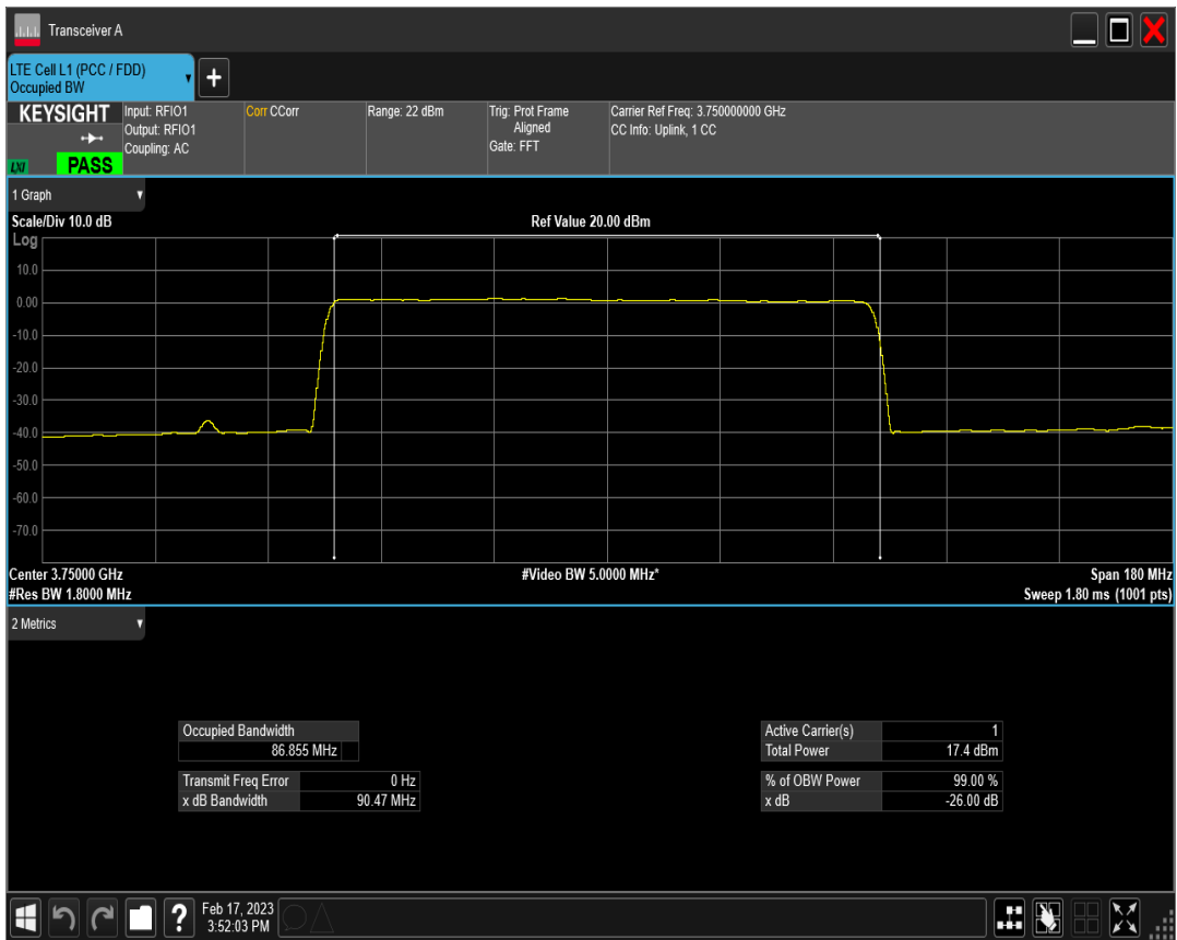
n78(3700-3800) SCS=30kHz DFT 256QAM BW=90MHz Channel=650000 RB=240@0
