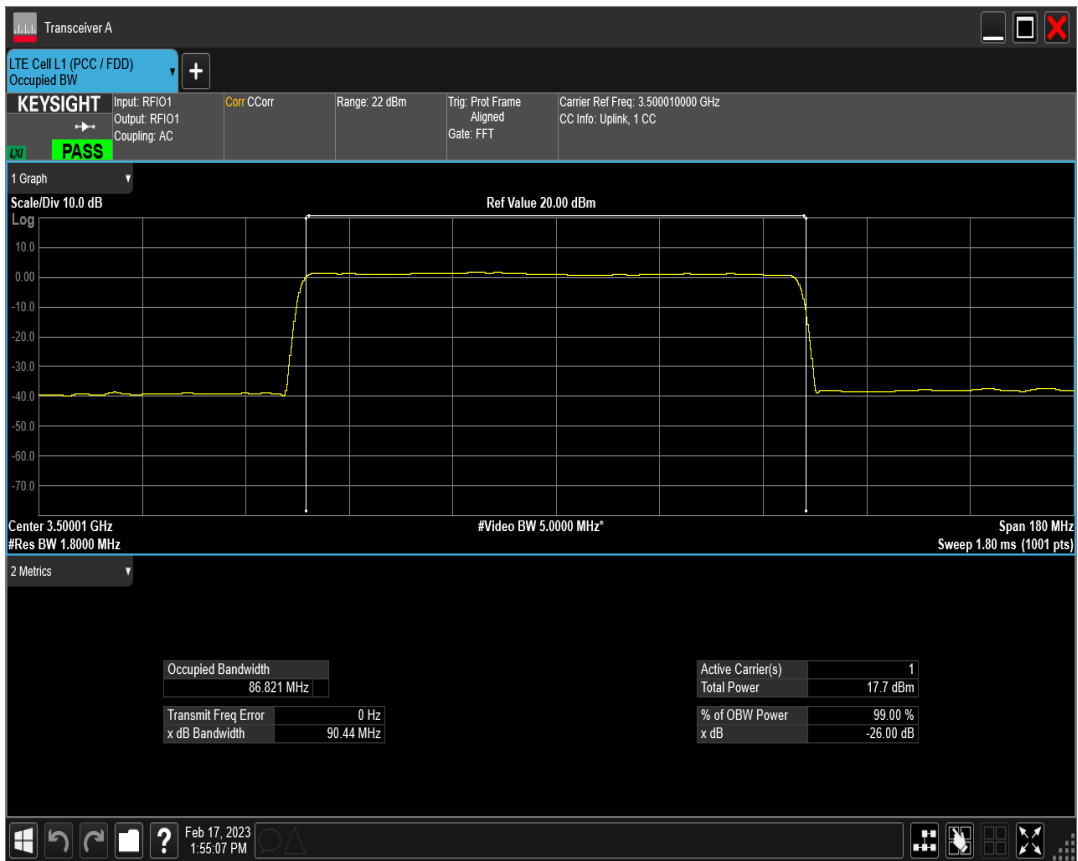
n78(3450-3550) SCS=30kHz DFT 64QAM BW=90MHz Channel=633334 RB=240@0
