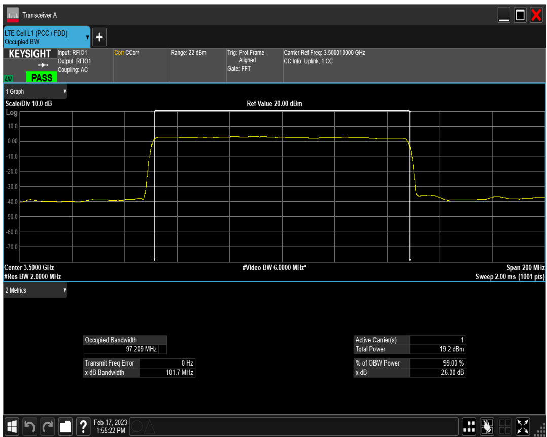
n78(3450-3550) SCS=30kHz DFT QPSK BW=100MHz Channel=633334 RB=270 @0
