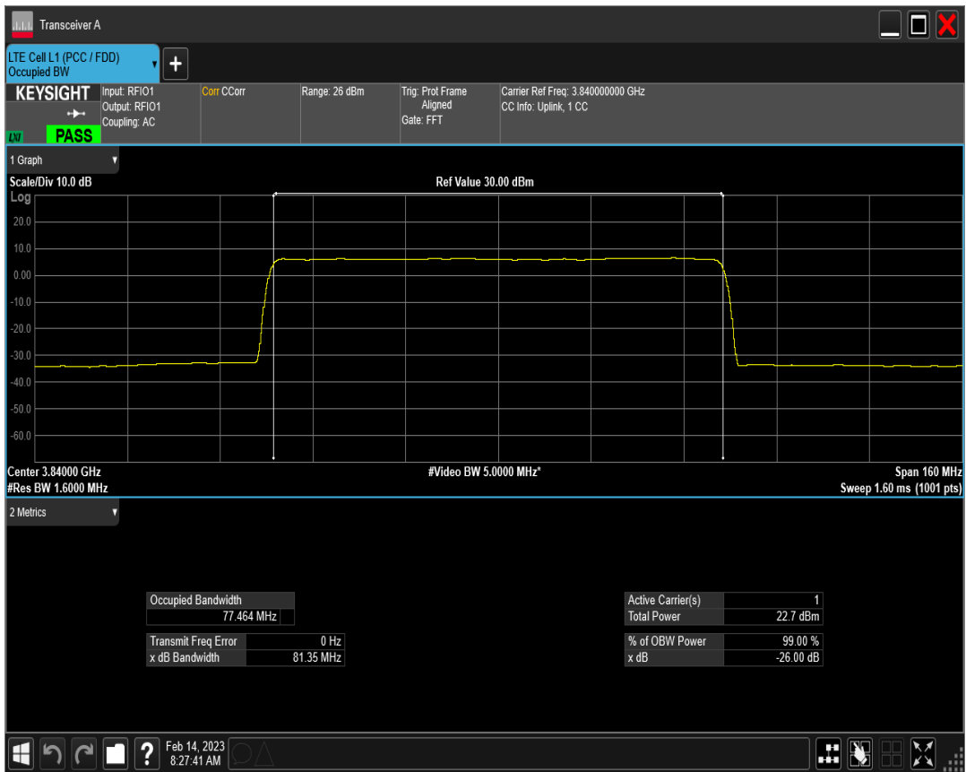
n77(3700-3980) SCS=30kHz DFT_QPSK BW=80MHz Channel=662666 RB=216@0
