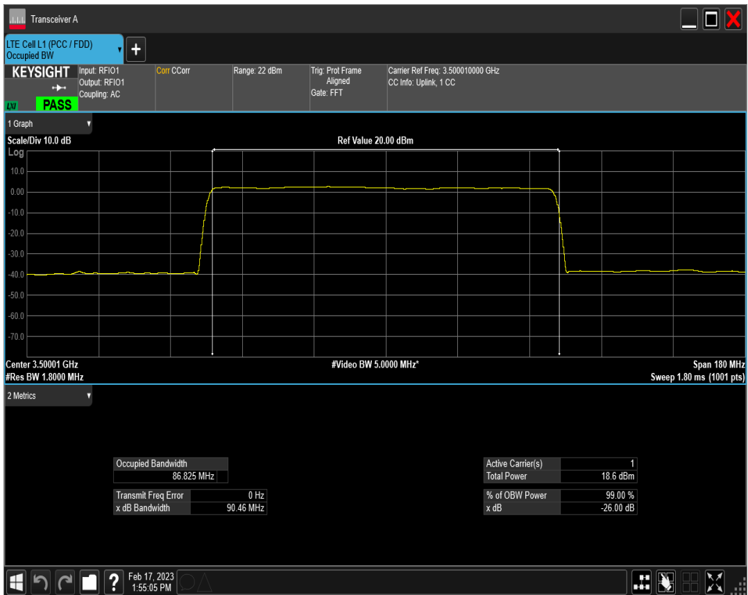
n78(3450-3550) SCS=30kHz DFT 16QAM BW=90MHz Channel=633334 RB=240@0
