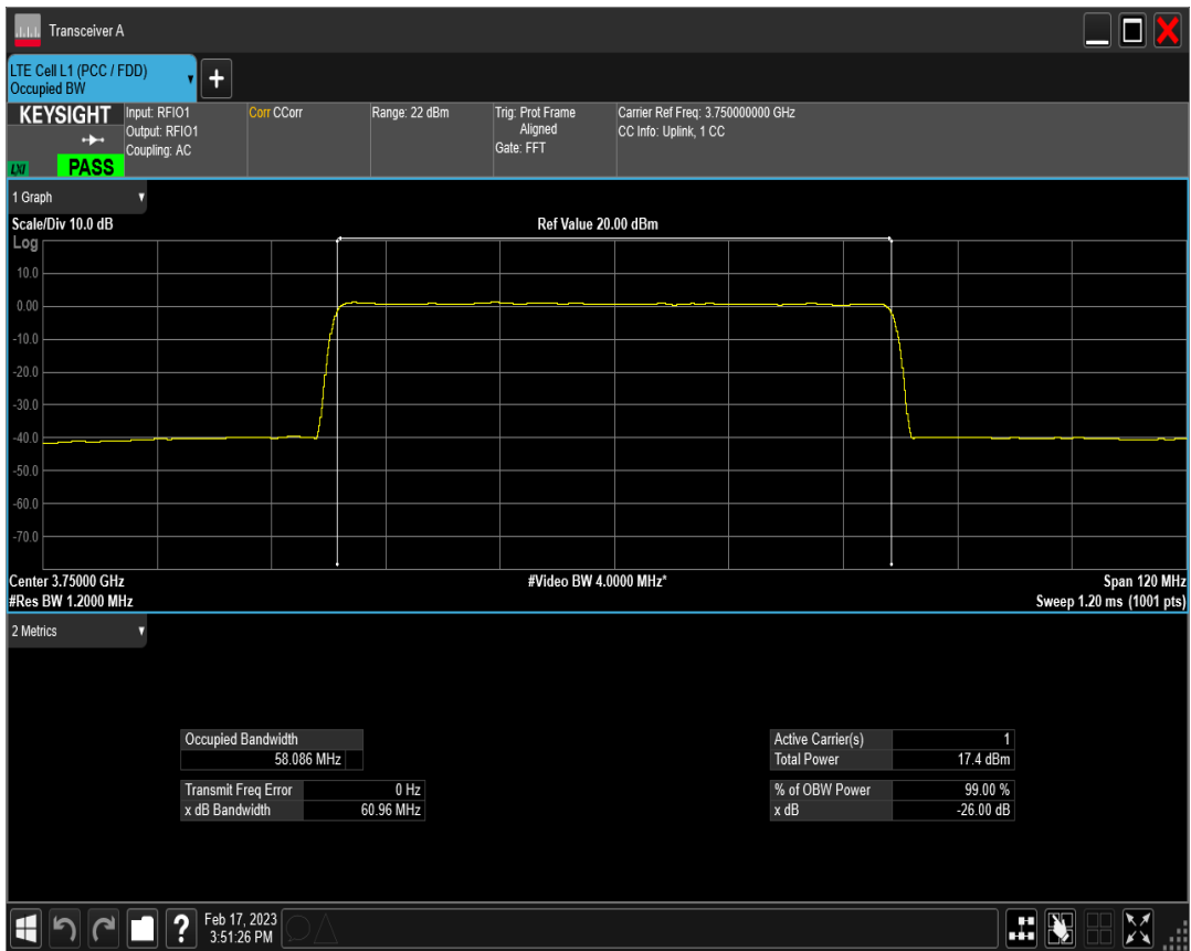
n78(3700-3800) SCS=30kHz DFT 256QAM BW=60MHz Channel=650000 RB=162@0
