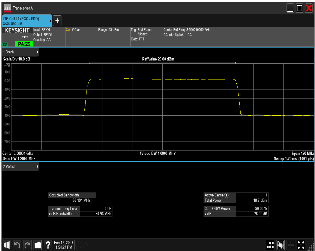
n78(3450-3550) SCS=30kHz DFT 16QAM BW=60MHz Channel=633334 RB=162@0
