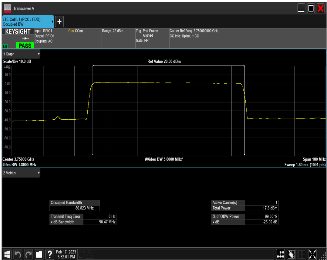
n78(3700-3800) SCS=30kHz DFT 64QAM BW=90MHz Channel=650000 RB=240@0
