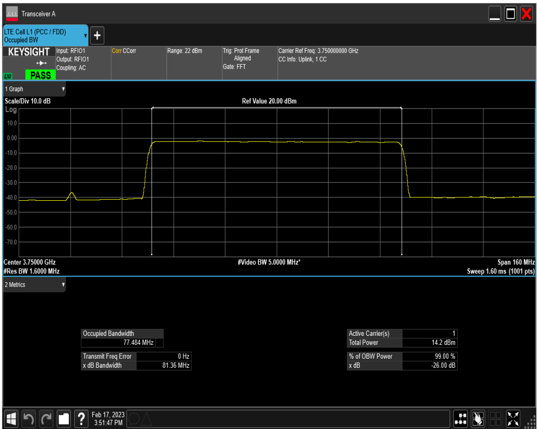
n78(3700-3800) SCS=30kHz DFT BPSK BW=90MHz Channel=650000 RB=240@0
