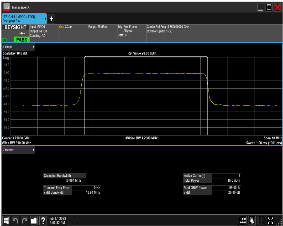
n78(3700-3800) SCS=30kHz DFT BPSK BW=40MHz Channel=650000 RB=100@0
