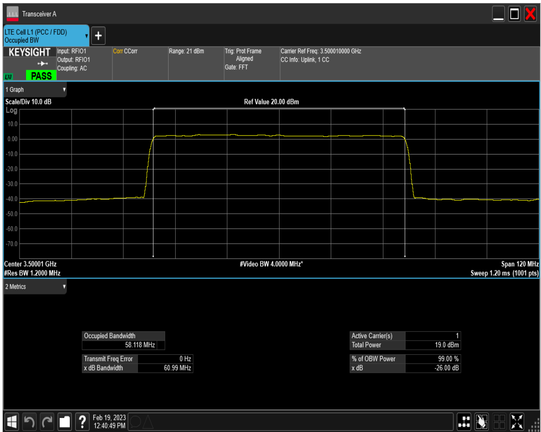
n78(3450-3550) SCS=30kHz DFT QPSK BW=60MHz Channel=633334 RB=162@0
