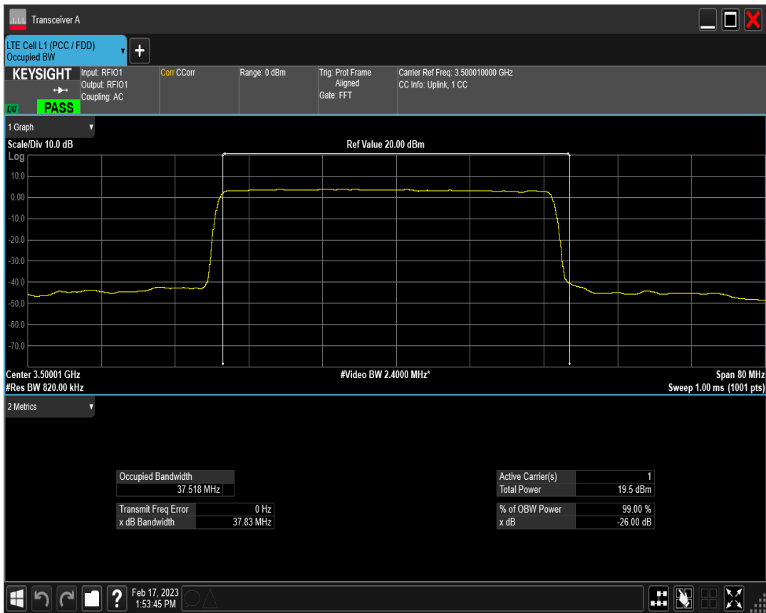
n78(3450-3550) SCS=30kHz DFT QPSK BW=40MHz Channel=633334 RB=100@0
