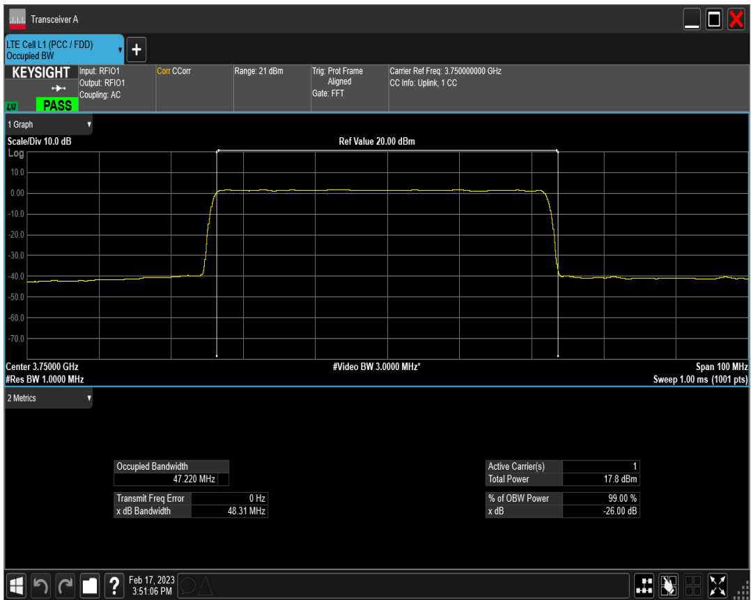
n78(3700-3800) SCS=30kHz DFT 64QAM BW=50MHz Channel=650000 RB=128@0
