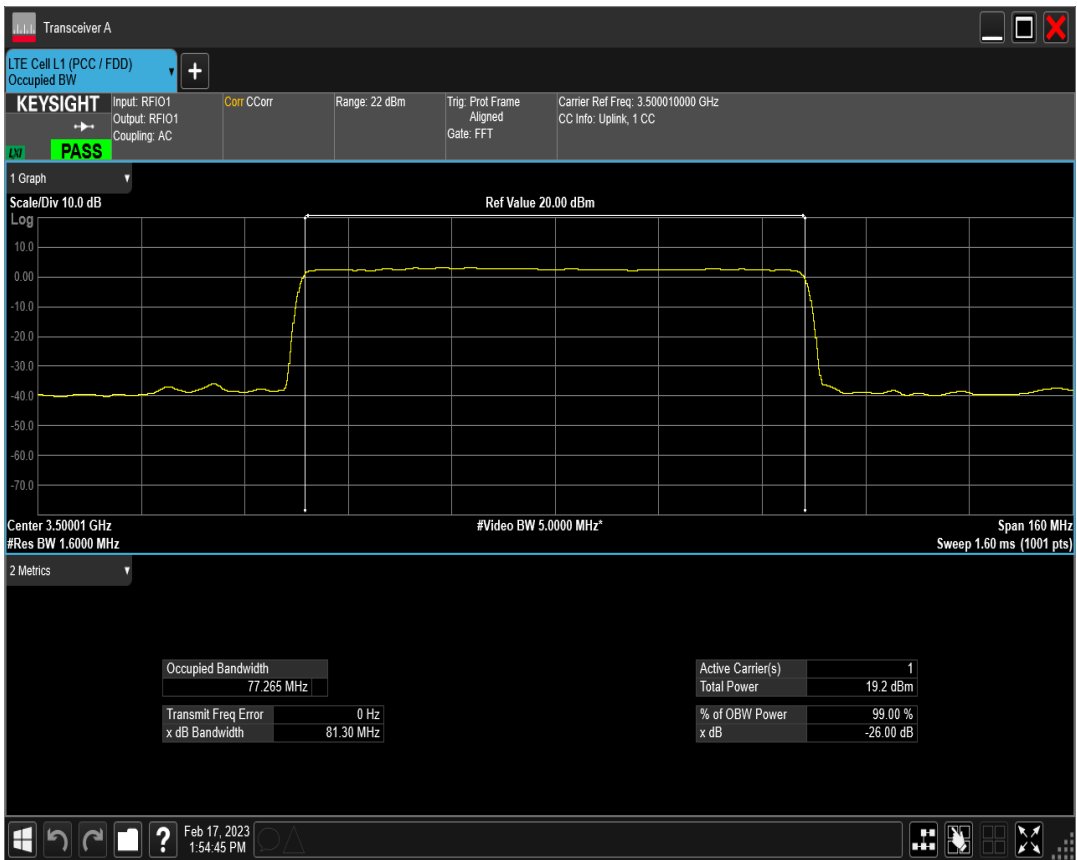
n78(3450-3550) SCS=30kHz DFT QPSK BW=80MHz Channel=633334 RB=216@0
