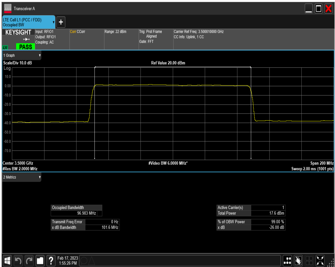
n78(3450-3550) SCS=30kHz DFT 64QAM BW=100MHz Channel=633334 RB=270@0
