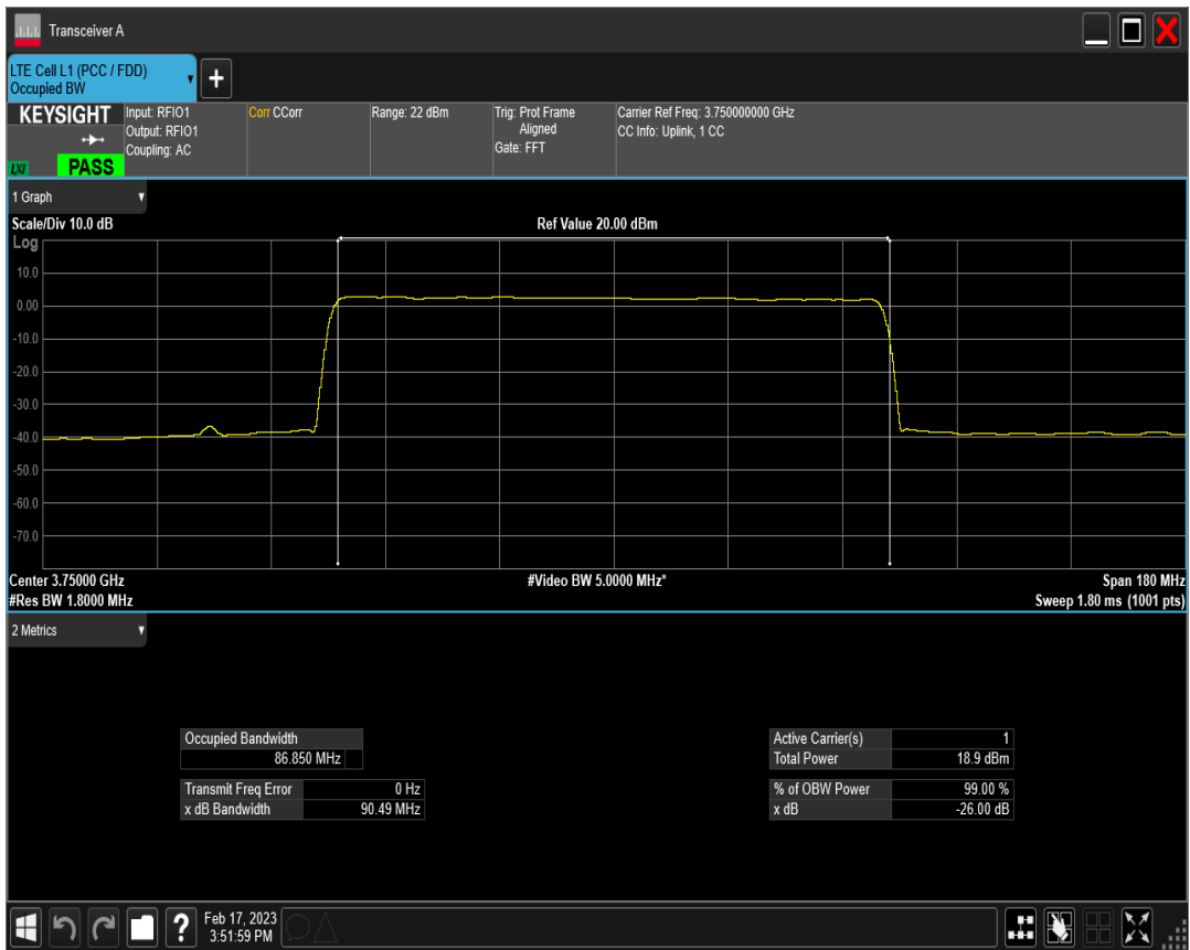
n78(3700-3800) SCS=30kHz DFT 16QAM BW=90MHz Channel=650000 RB=240@0
