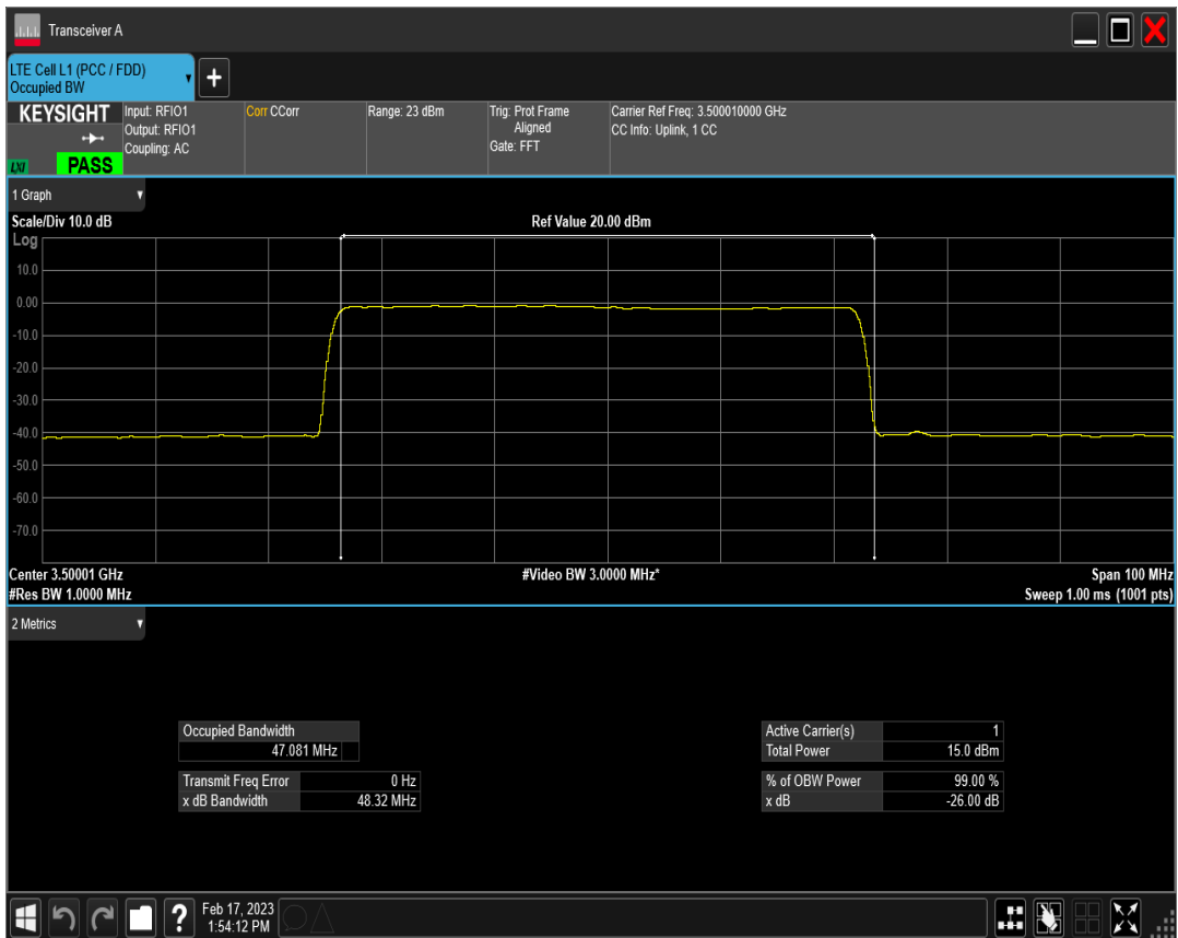
n78(3450-3550) SCS=30kHz DFT BPSK BW=60MHz Channel=633334 RB=162@0
