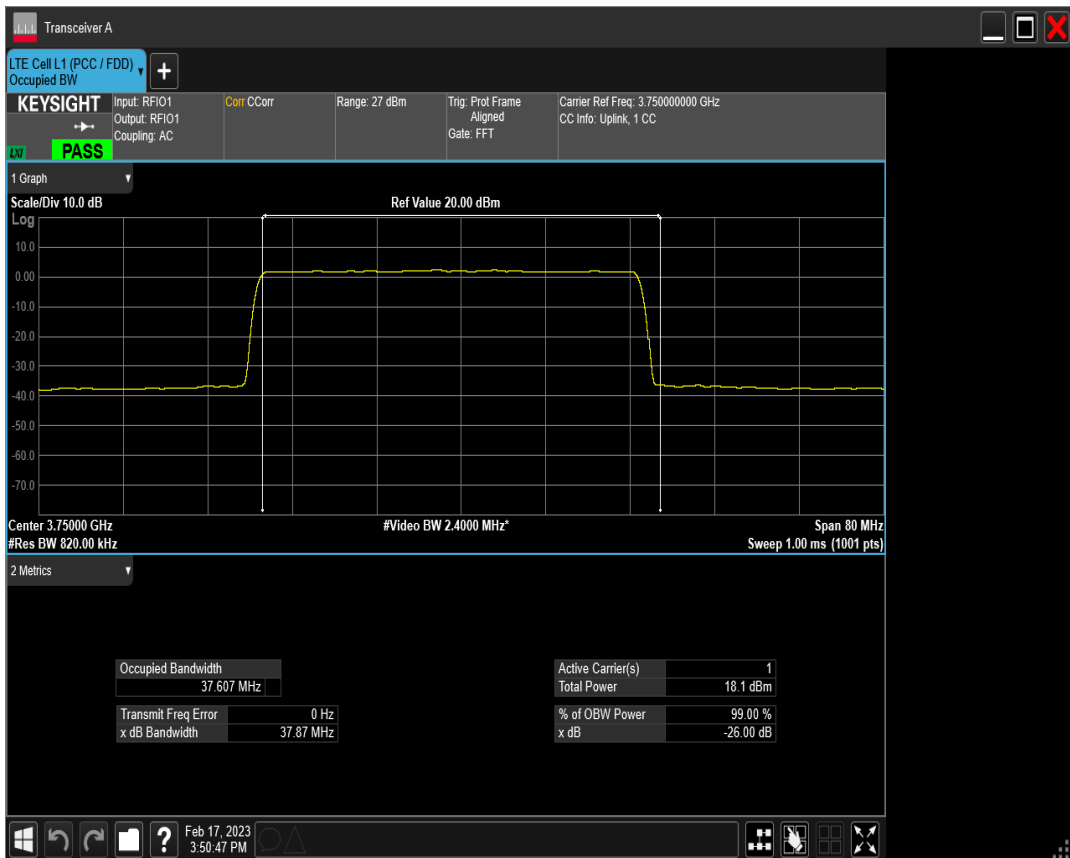
n78(3700-3800) SCS=30kHz DFT 64QAM BW=40MHz Channel=650000 RB=100@0
