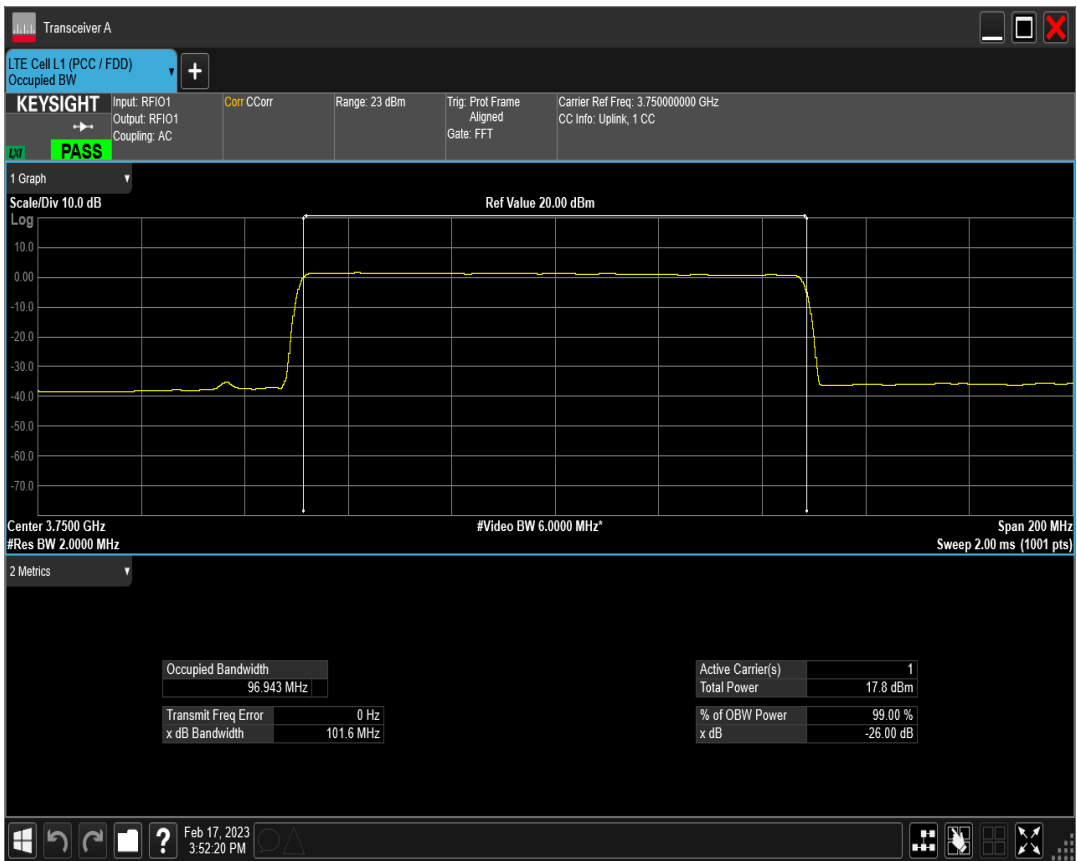
n78(3700-3800) SCS=30kHz DFT 64QAM BW=100MHz Channel=650000 RB=270@0
