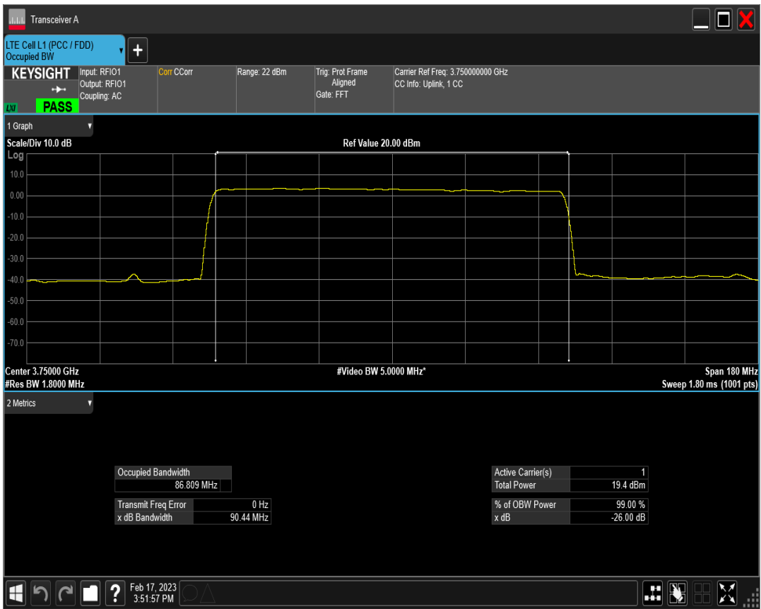
n78(3700-3800) SCS=30kHz DFT QPSK BW=90MHz Channel=650000 RB=240@0
