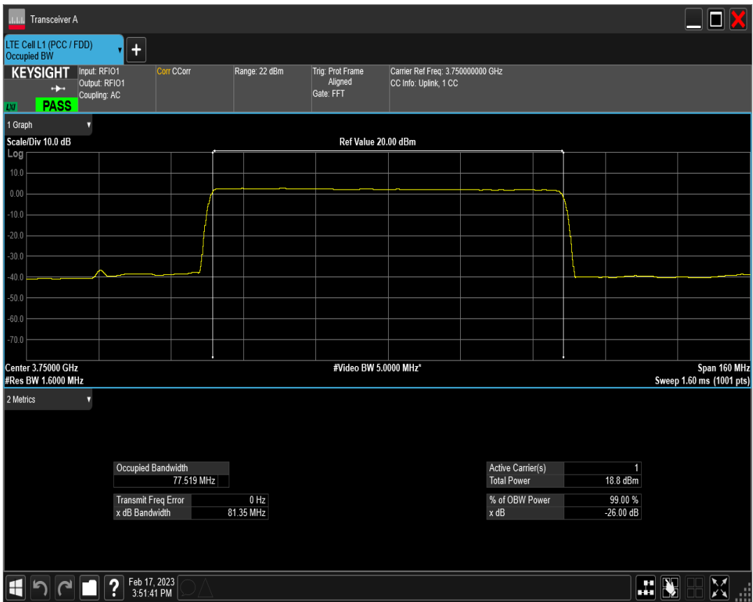
n78(3700-3800) SCS=30kHz DFT 16QAM BW=80MHz Channel=650000 RB=216@0
