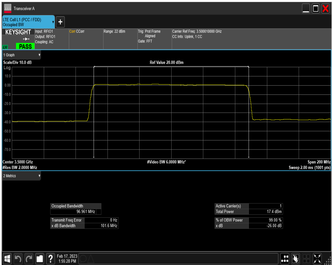
n78(3450-3550) SCS=30kHz DFT 256QAM BW=100MHz Channel=633334 RB=270@0
