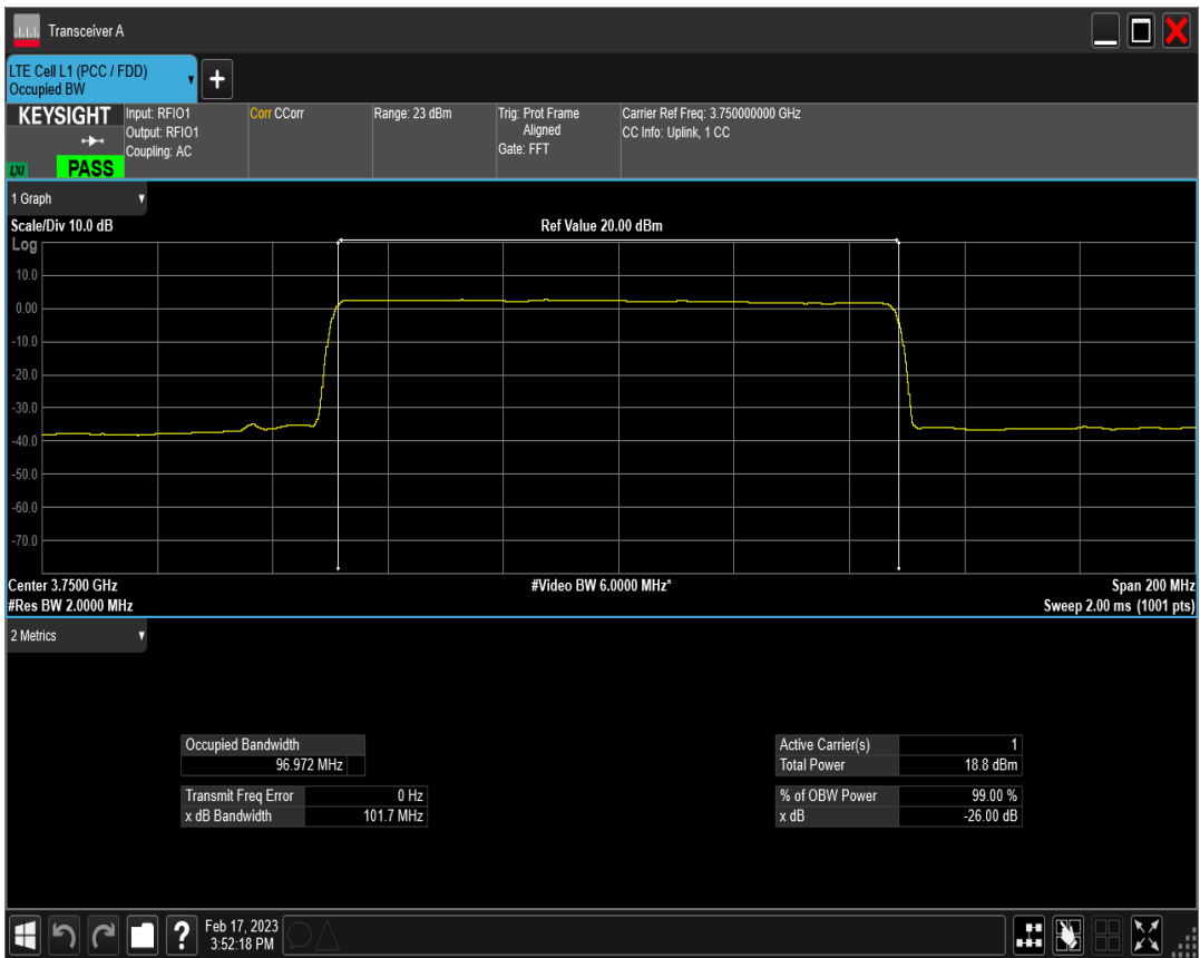
n78(3700-3800) SCS=30kHz DFT 16QAM BW=100MHz Channel=650000 RB=270@0
