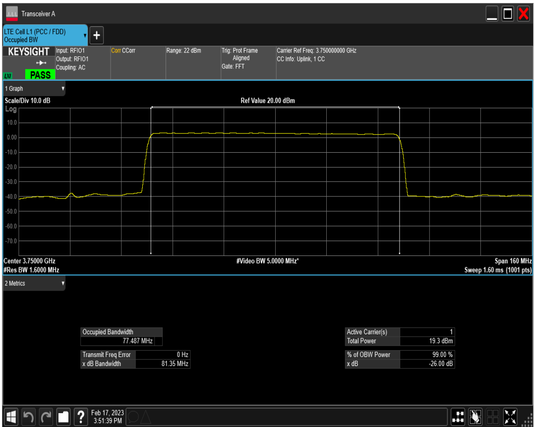
n78(3700-3800) SCS=30kHz DFT QPSK BW=80MHz Channel=650000 RB=216@0
