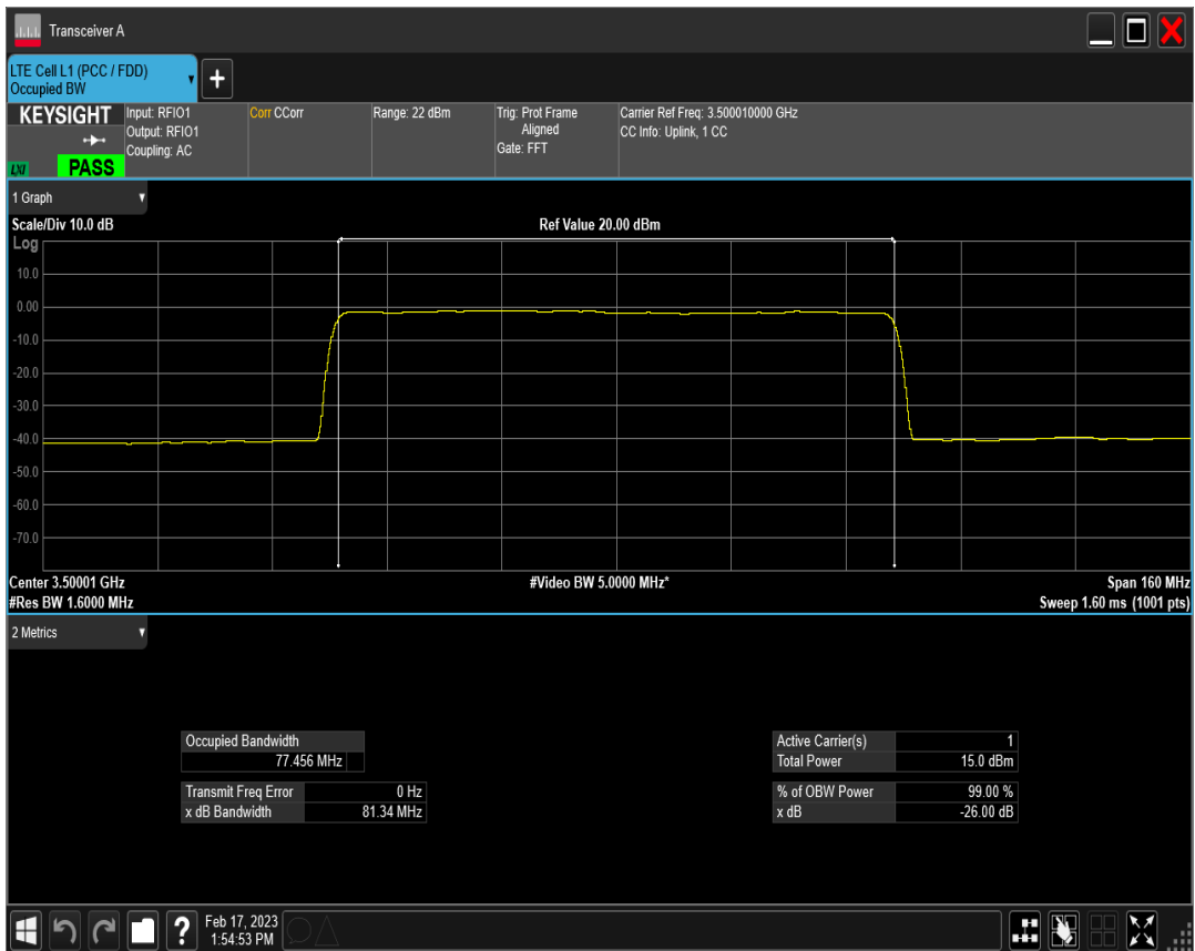
n78(3450-3550) SCS=30kHz DFT BPSK BW=90MHz Channel=633334 RB=240@0
