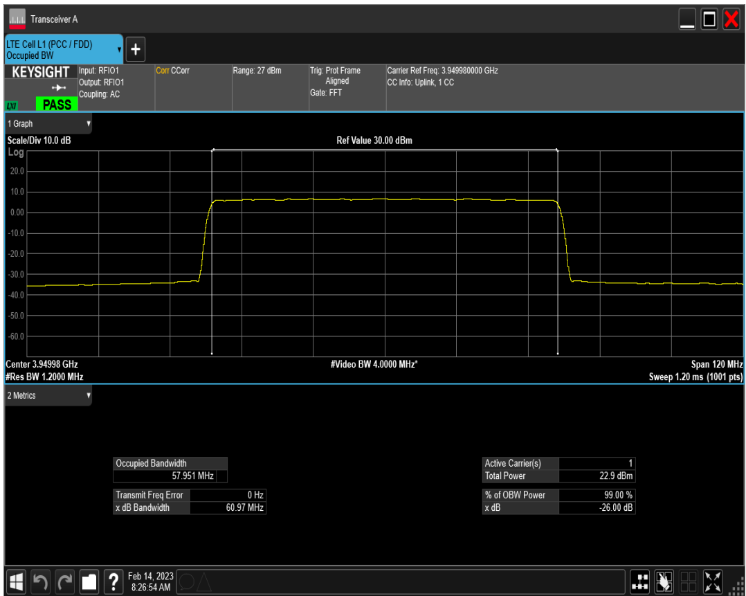
n77(3700-3980) SCS=30kHz DFT_QPSK BW=80MHz Channel=649334 RB=216@0
