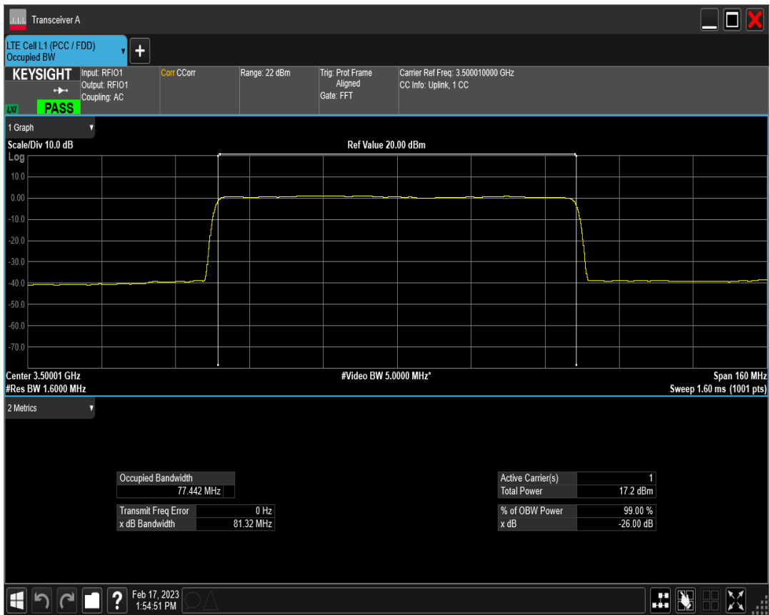
n78(3450-3550) SCS=30kHz DFT 256QAM BW=80MHz Channel=633334 RB=216@0
