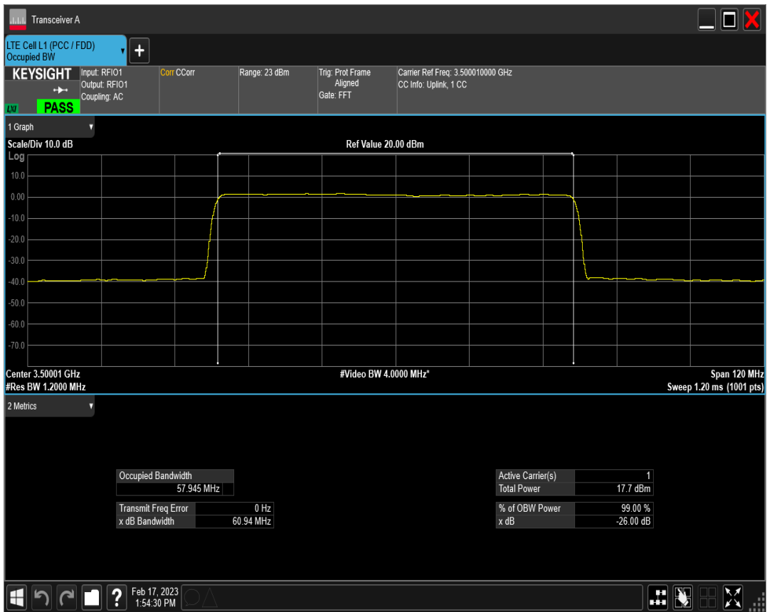
n78(3450-3550) SCS=30kHz DFT 64QAM BW=60MHz Channel=633334 RB=162@0
