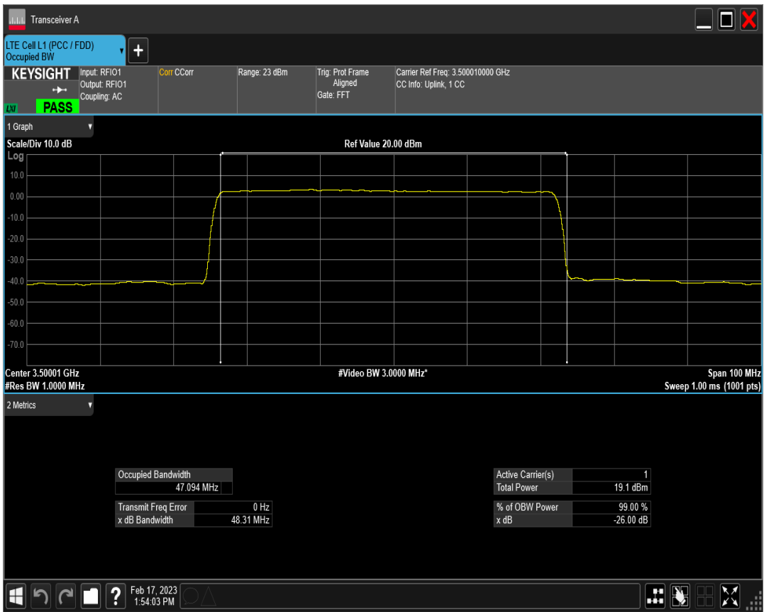
n78(3450-3550) SCS=30kHz DFT QPSK BW=50MHz Channel=633334 RB=128@0
