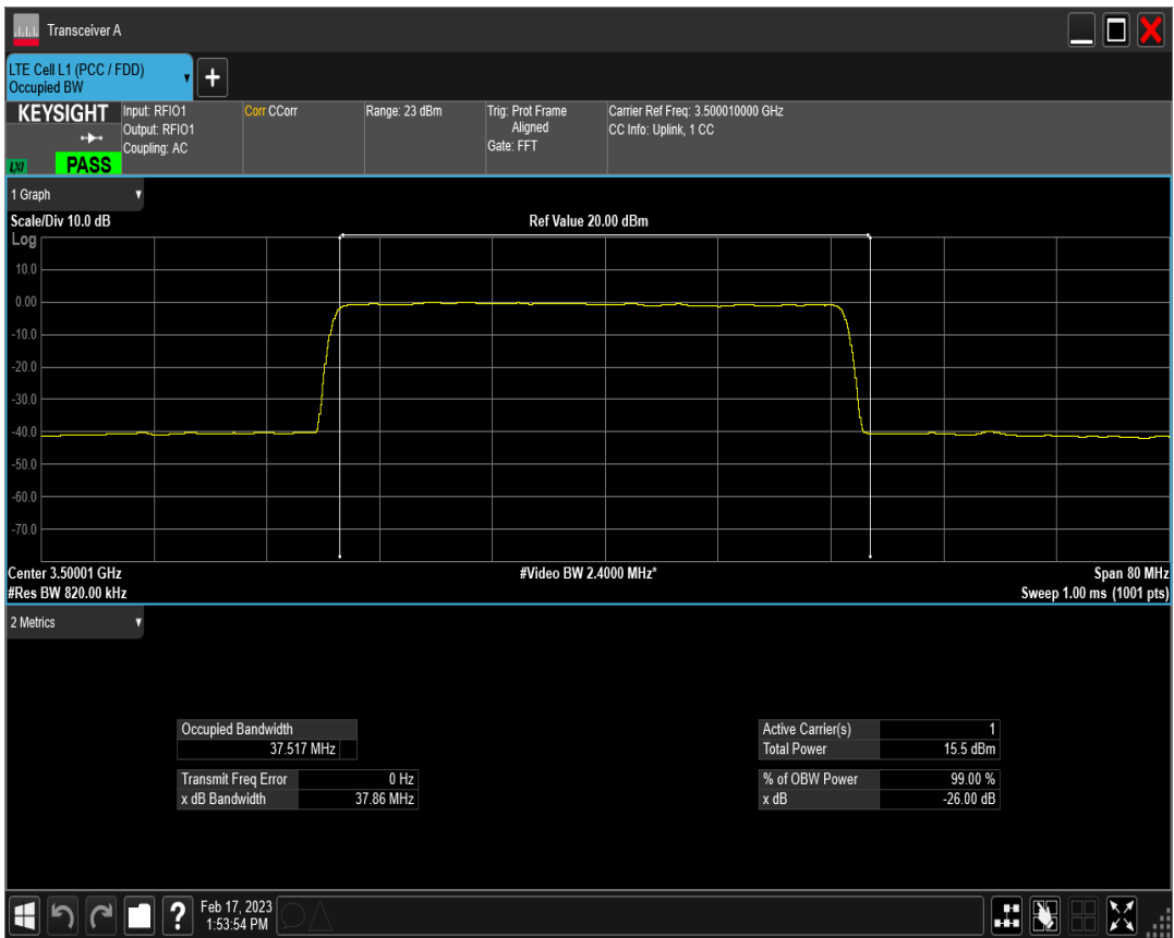
n78(3450-3550) SCS=30kHz DFT BPSK BW=50MHz Channel=633334 RB=128@0
