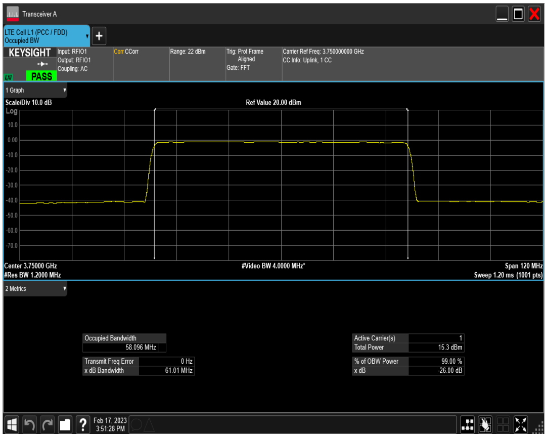
n78(3700-3800) SCS=30kHz DFT BPSK BW=80MHz Channel=650000 RB=216@0
