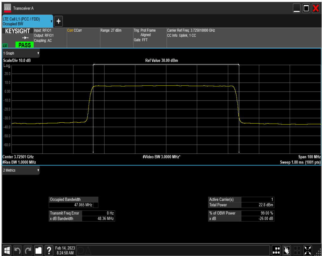
n77(3700-3980) SCS=30kHz DFT_QPSK BW=50MHz Channel=656000 RB=128@0
