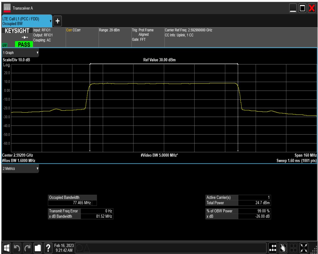
n41 SCS=30kHz DFT_QPSK BW=80MHz Channel=529998 RB=216@0
