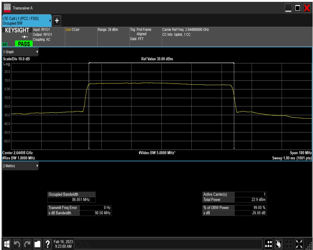
n41 SCS=30kHz DFT_QPSK BW=100MHz Channel=509202 RB=270@0
