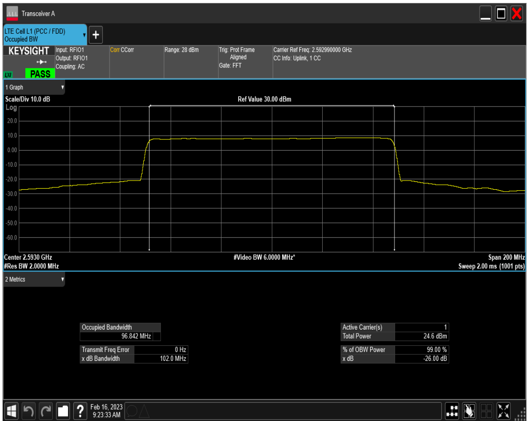
n41 SCS=30kHz DFT_QPSK BW=100MHz Channel=528000 RB=270@0
