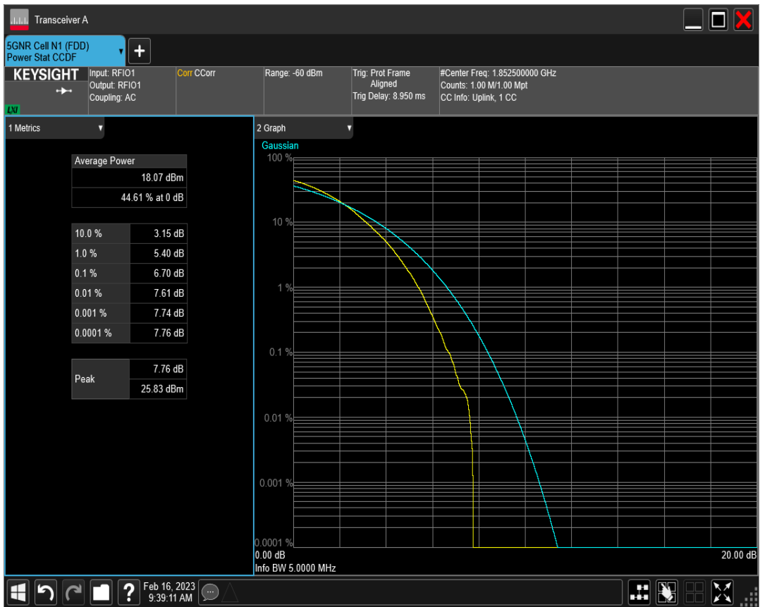
n2 SCS=15kHz DFT_QAM256 BW=5MHz Channel=376000 RB=25@0
