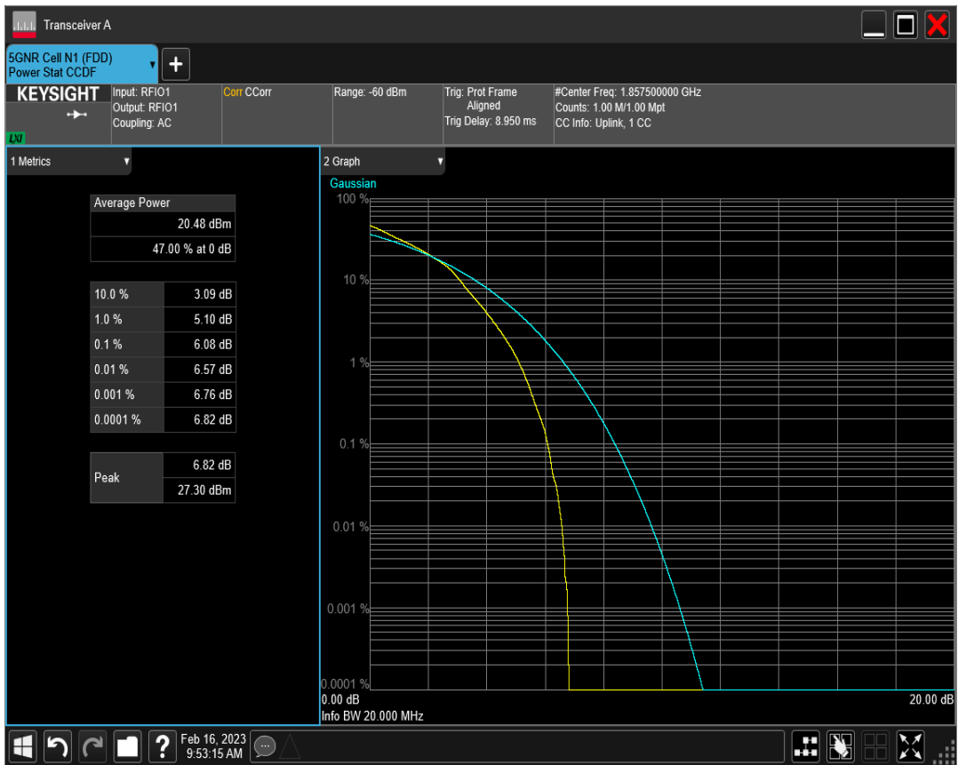
n2 SCS=15kHz DFT_QAM16 BW=15MHz Channel=376000 RB=75@0
