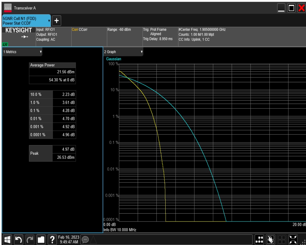
n2 SCS=15kHz DFT_BPSK BW=15MHz Channel=371500 RB=75@0
