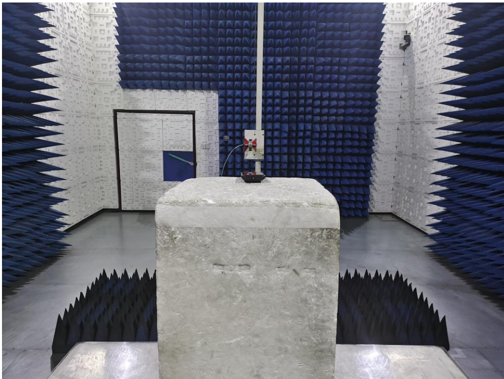
RADIATED EMISSION TEST SETUP ABOVE 1GHz
