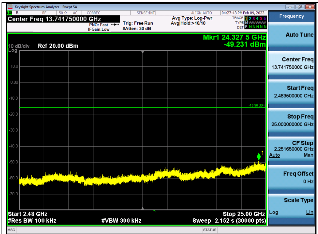
Test_Graph_EDR_ANT1_2441_2Mbps_Higher Band Emissions
