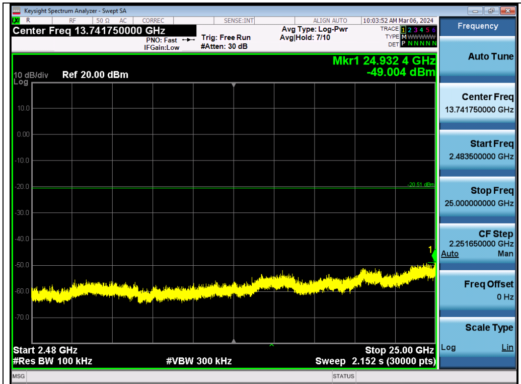
Test_Graph_LE2M_ANT1_2440_2Mbps_Higher Band Emissions
