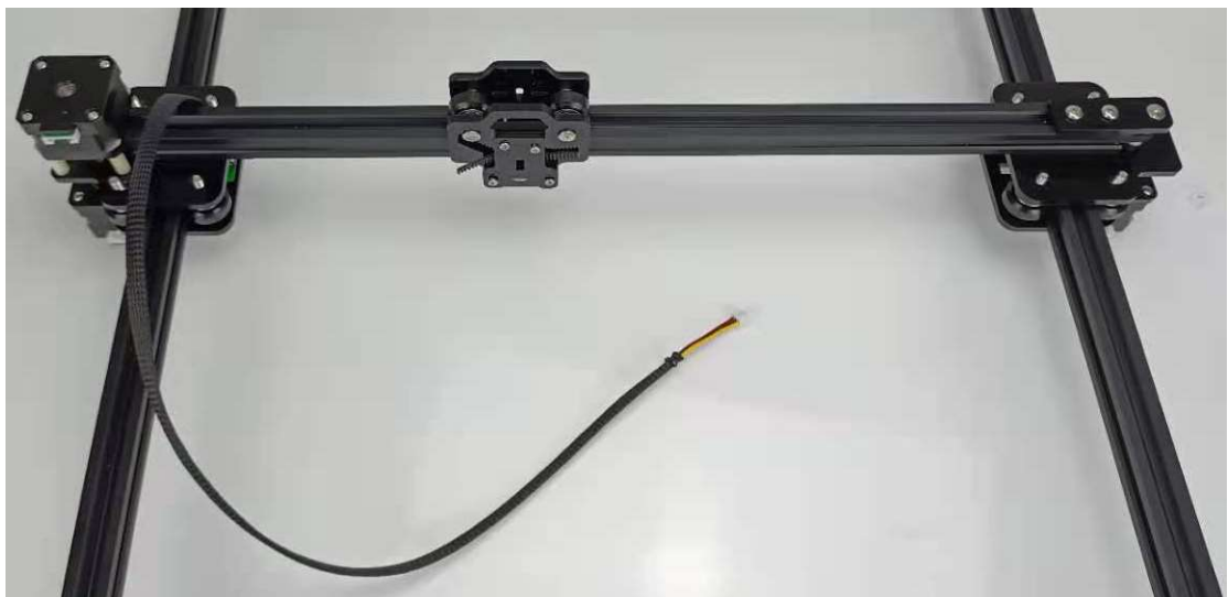
8. Install and fix x and y axis wires
