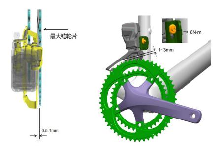
Use a 5mm Allen wrench to attach the front derailleur to the lugs and tighten the mounting bolts. When adjusting the mounting position, make sure that the plane of the outer guide plate is directly above the largest chainring, and the distance
