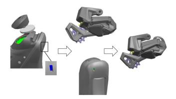
3. Hand change pairing: Unscrew the left/right hand battery cover screws and remove the battery cover. Put on the battery to enter pairing mode, and the blue indicator flashes. After successfully pairing with the rear derailleur, the rear derailleur and left/right hand change indicator will light up green for 1 second, and the blue indicator of the rear derailleur will continue to flash. Then follow the same steps with the rest of the hand.
