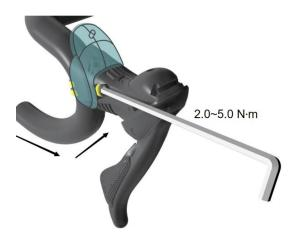
Flip open the rubber sleeve from the top end, loosen the set screws with a 5mm Allen wrench, and then thread the clamp ring through the handlebar. Attach the handset to the handlebar and tighten the fixing bolts.
