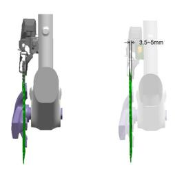
Use the right-hand variable to make fine adjustments until the front derailleur inner guide fits snugly against the chain of the largest chain. If there is no chain as a
