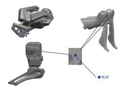
4. Exit pairing: After pairing the two hand changes, front dial and back dial one by one, press the left/right hand change any button to exit the pairing mode. The device that has been successfully paired flashes 5 times with a blue light.
