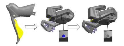
After the fine-tuning is completed, press and hold the left hand for 3 seconds to exit the fine-tuning.
