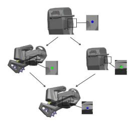
2. Front dial pairing: Open the front dial dust cover, connect the magnetic connector of the charging cable connected to the power supply with the magnetic connector of the front dial, and the indicator flashes blue to enter the pairing mode. After successfully pairing with the rear dial, the rear and front dial indicators will light up green for 1 second, while the blue indicator will continue to flash after the rear dial.
