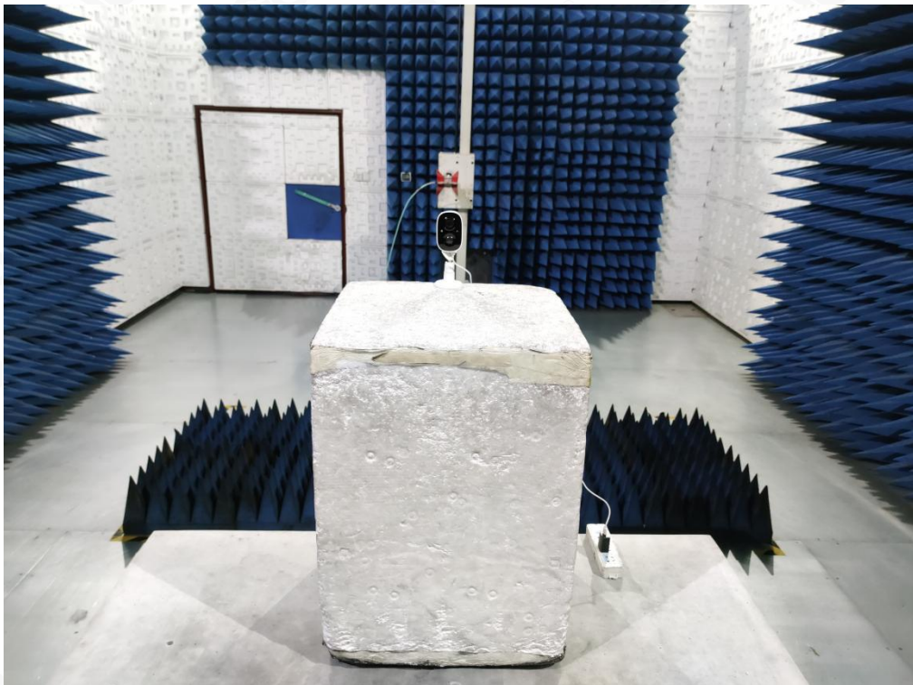
FCC RADIATED EMISSION TEST SETUP ABOVE 1GHZ
