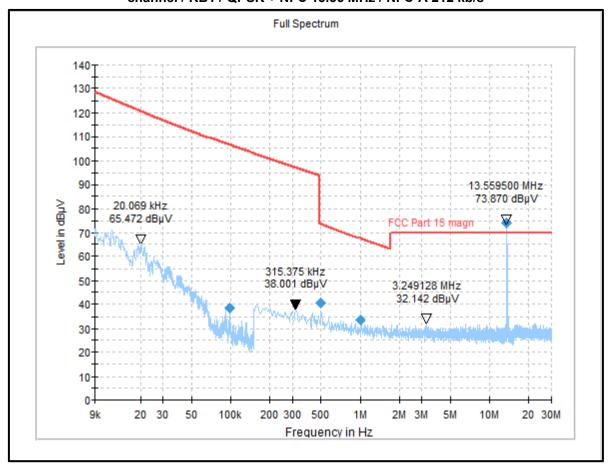
Note: The emission at 13.56 MHz is from NFC and we cannot de-activate it during the measurement.
