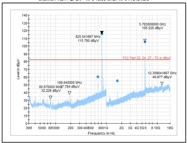
Note: The peak at 825.04 MHz is the uplink frequency of the respective cellular band tested. Note: The peak at 5783.00 MHz is the frequency of the WIFI band tested.
