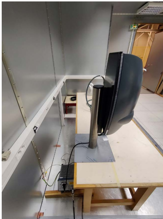
conducted emission set-up (0.15-30MHz)
