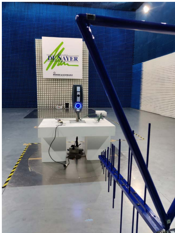
Spurious emission set-up (30-1000MHz) 3m
