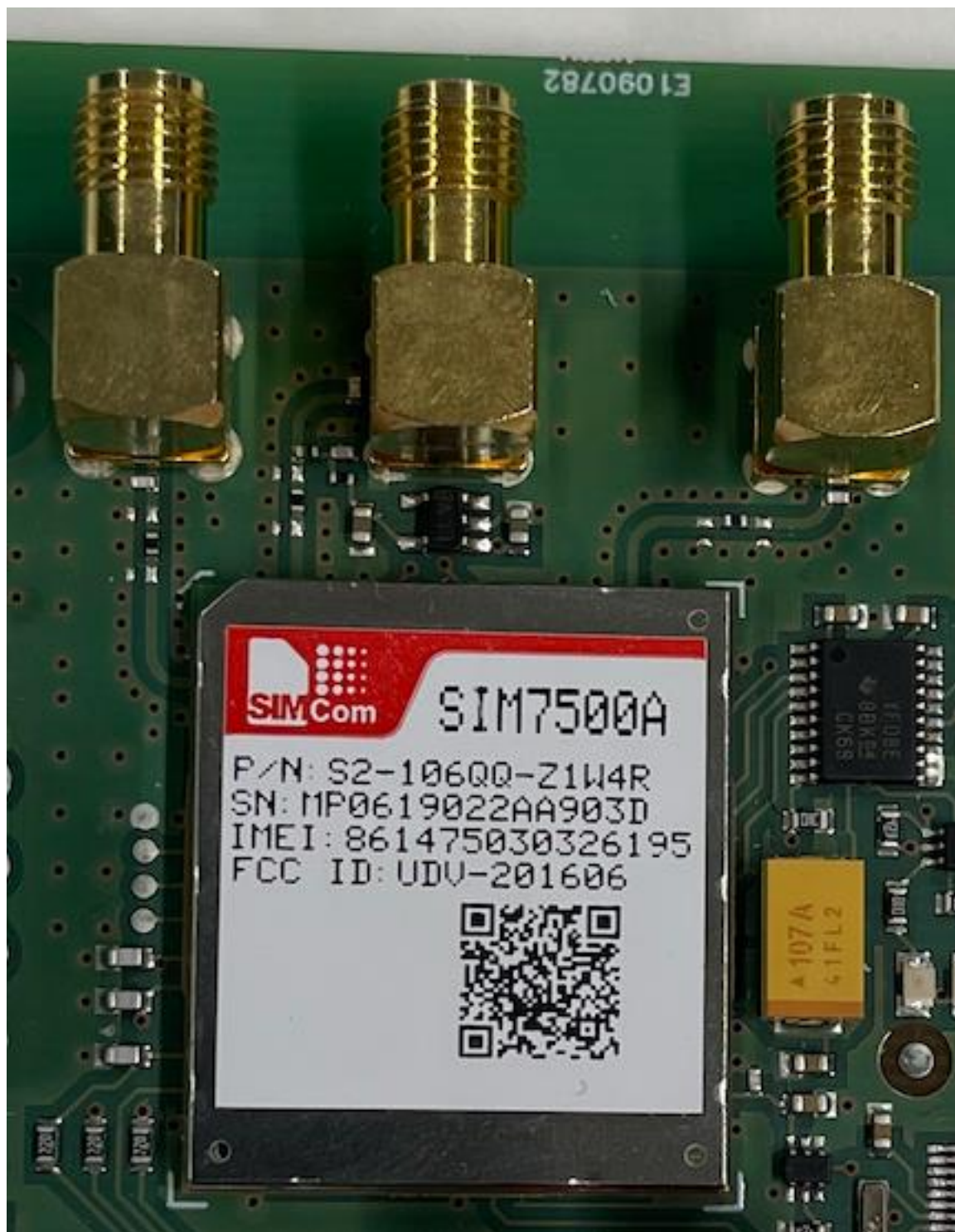
LTE PCB view, front side, zoom in to the transmitter part
