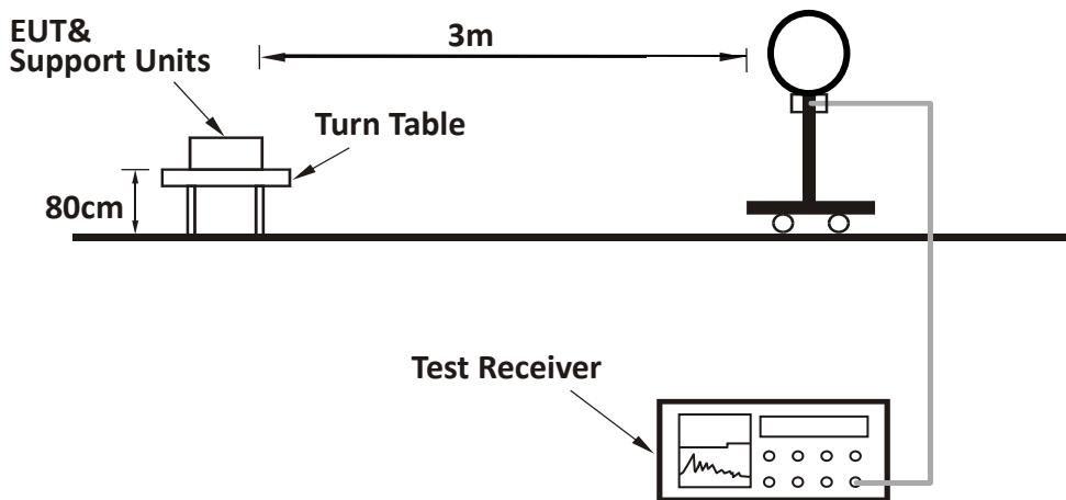
**For Radiated emission 30MHz to 1GHz:**
