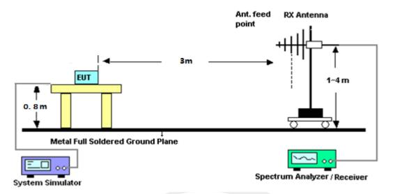
For radiated test from above 1GHz
