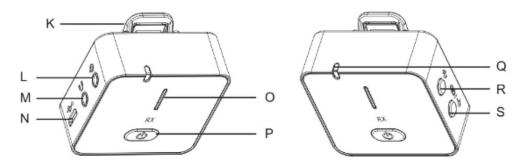
K: Fixing clip: can be quickly installed to the required fixed position.
