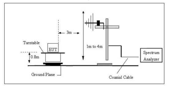
(C) Radiated Emission Test-Up Frequency Above 1GHz
