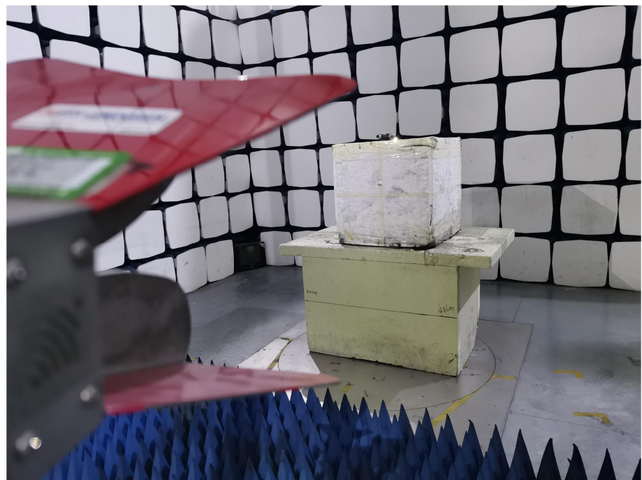
Radiation Emission Test Setup (1GHz to 18GHz)
