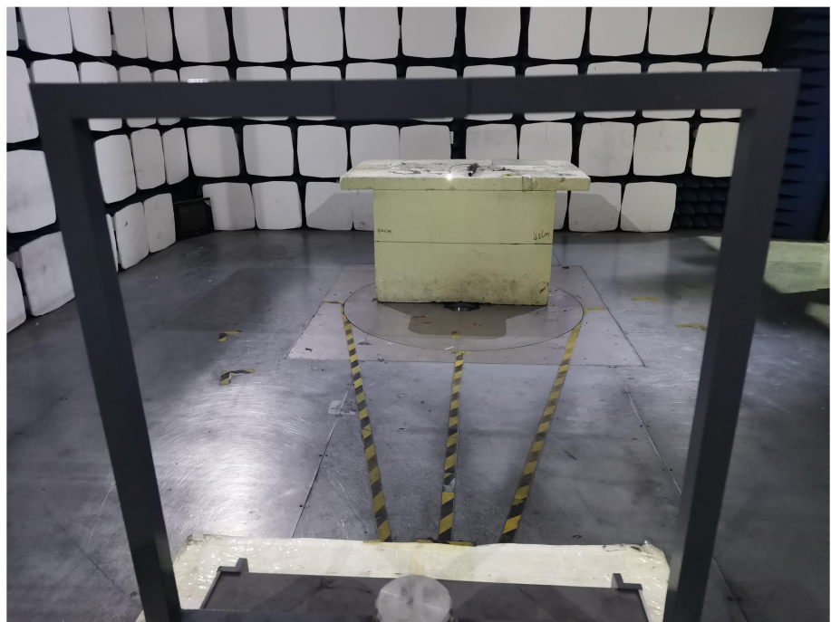
Radiation Emission Test Setup (Below 30MHz)
