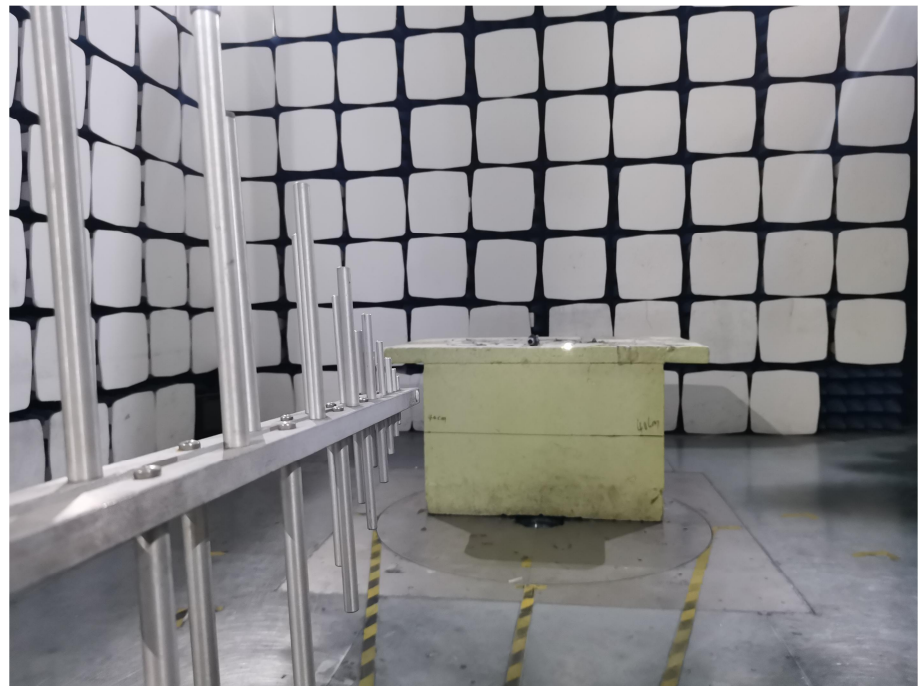
Radiation Emission Test Setup (30MHz to 1GHz)
