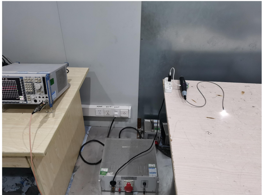
Conducted Emission Test Setup
