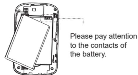
4. After inserting SIM and battery correctly, press power switch about 5 seconds to boot it, it can be used normally.
