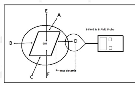
Note: Due to installation limitations no tests from the underside of the charging device (Test Position F) are required. The test position F is required when the distance is 0 cm for partable device.
