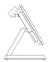
Dual-screen Device15+10.4 W x D x H: 349 x 320 x 331, Main Display flip angle :5-50°, second display flip angle: 0-25°
