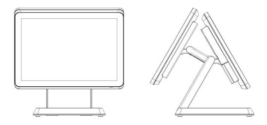
Dual-screen 15+15 Device, W x D x H: 349 x 331 x 345mm, Main Display flip angle :5-50 $^{\circ}$  , second display flip angle: 0-30 $^{\circ}$
